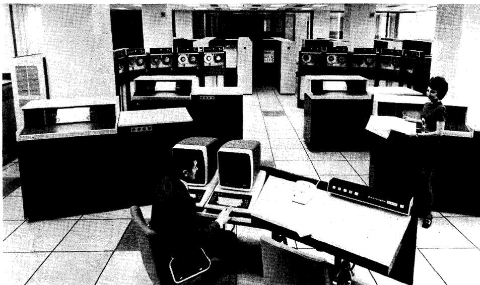
*B 6700 systems, now available in 14 different models, can include as many as 3 central processors, 3 input/output processors, and 6 million bytes of core storage. The dual-display operator console permits convenient communication with the Master Control Program that schedules and controls all B 6700 operations.*
