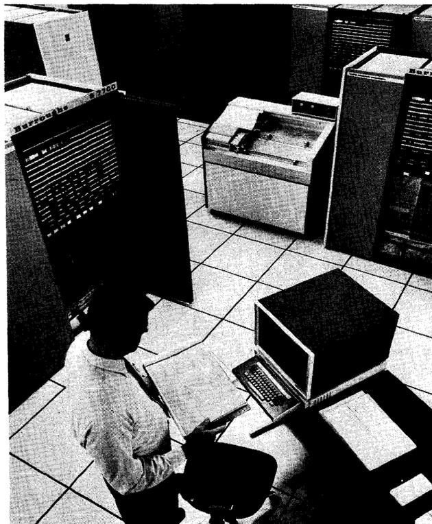
*The B 7700 is the largest and most advanced computer in Burroughs' broad "700 Systems" product line. The B 7700 central exchange can accommodate up to 6 million bytes of core storage and a total of up to 8 central processors and input/output processors.*
