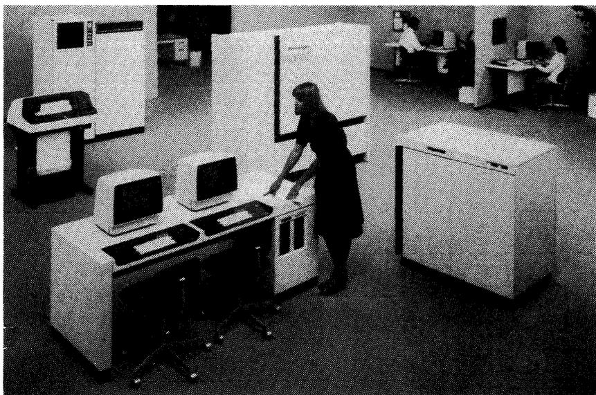
The Burroughs B 5930 system includes a central processing unit, 1.5 to 6.2 million bytes of main memory, a dual-display operator console, and support for a line printer, a magnetic tape subsystem, and two disk pack subsystems. The system utilizes Burroughs' new multi-level Function Processor architecture.
