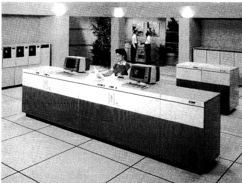
*The Burroughs A 10 H is an intermediate-range, dual-processor mainframe with up to 96 megabytes of main memory, two I/O cabinets with a maximum of 80 DLPs, and up to 288 data communication lines.*
