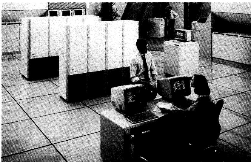
*Burroughs' A 15 large-scale computer series features Emitter Coupled Logic gate array technology and 24M bytes of main memory expandable to 192M bytes. The A 15 is available in eight models ranging from one to four central processors.*
