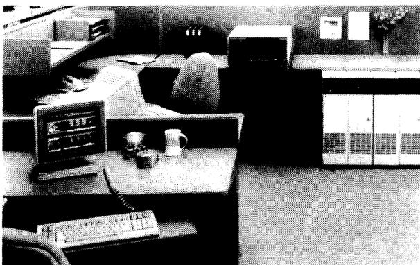
*The XE550 marks Burroughs' entry into the Unix-based computer market. Based on Centix, an enhanced version of Unix System V, the XE550 can reportedly run currently available Unix System V applications. The XE550, built around a multiprocessor architecture, supports up to 12MB of memory, up to 1.3GB of disk storage, and up to 32 users.*
