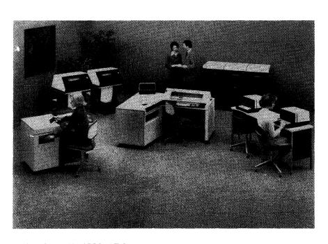
The BSM drive is a new double-density floppy drive capable of reading and writing floppy disks on both sides by means of two sets of read/write heads. The BSM is also available in a single or dual stand-alone configuration. The console printer may be either a 60-cps dot matrix printer or a newly developed 180-cps dot matrix printer. The new printer offers three times the speed of the other unit as well as up to three independent pin-feed forms advance units.
