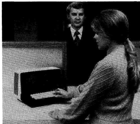
*The Self-Scan display panel is an integral part of many peripherals provided by Burroughs, including the new TD 730 display/keyboard. The panel provides 8 lines of 32 characters or 12 lines of 40 characters. Each character is presented in the form of a 5-by-7 dot matrix. In the TD 730, a memory of up to 4080 characters permits paging operations.*
