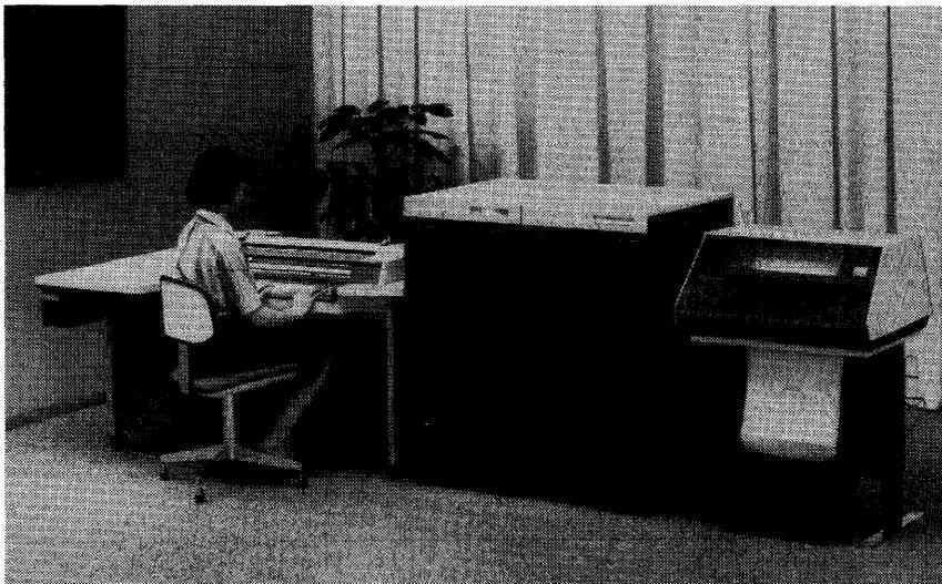
*This small B 730 configuration includes (from left to right) the system console, processor module, dual cartridge disk drive unit, and an 85-lpm printer. The system can be augmented with a variety of additional peripheral equipment.*
