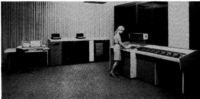
*The B 723 is a packaged system oriented toward banking and other financial applications. The system includes a system console, a dual-cartridge disk drive, a line printer, and a MICR reader/sorter (at right).*
