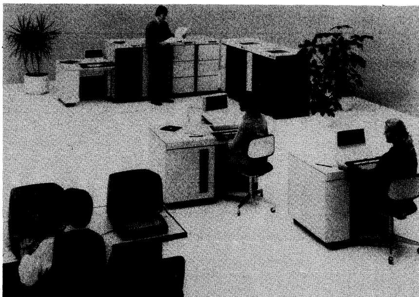
*This large configuration of the Burroughs B 820 system includes, in the foreground, two TD 830 CRT's at left, a Direct Data Entry Station (DDES) at right, and an AE 500 Audit Entry Station with two Super Mini-Disk drives in the center. From left to right in the background are the DDES console, a double-width B 820 processor, two disk pack drive cabinets, and two line printers.*
