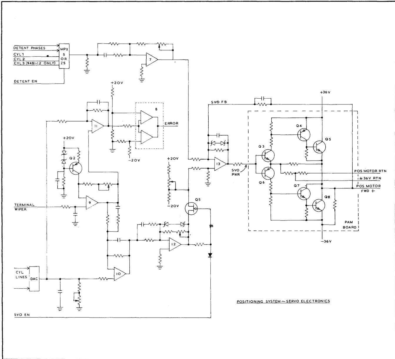
Figure 2-8. Positioning System Servo Electronics
