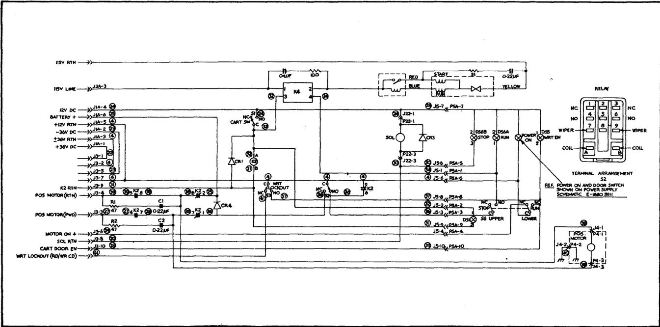
Figure 2-3. Main Harnesses, Switches And Relays.
