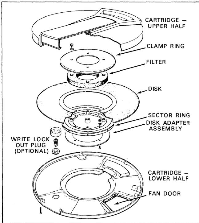
Figure 1-5. Disk Cartridge (Exploded View)
