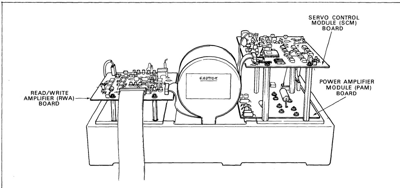
Figure 1-24. Rear View of Module Showing Boards (9480-12)
