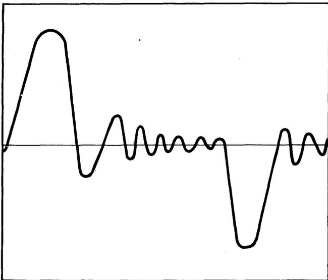
Figure 4-10b. Servo Offset Adjustment – Correct
