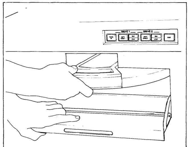
Figure 1-6. Inserting a Disk Cartridge into the Receiver (Upper Drive Module)
