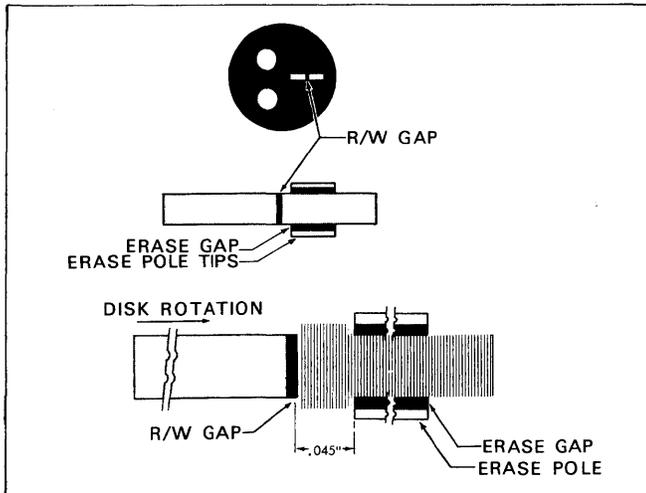
Figure 1-13. Head Recording Principles
