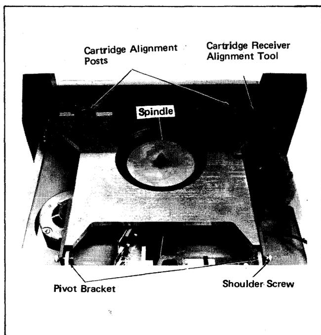
Figure 5-18. Receiver Alignment Tool
