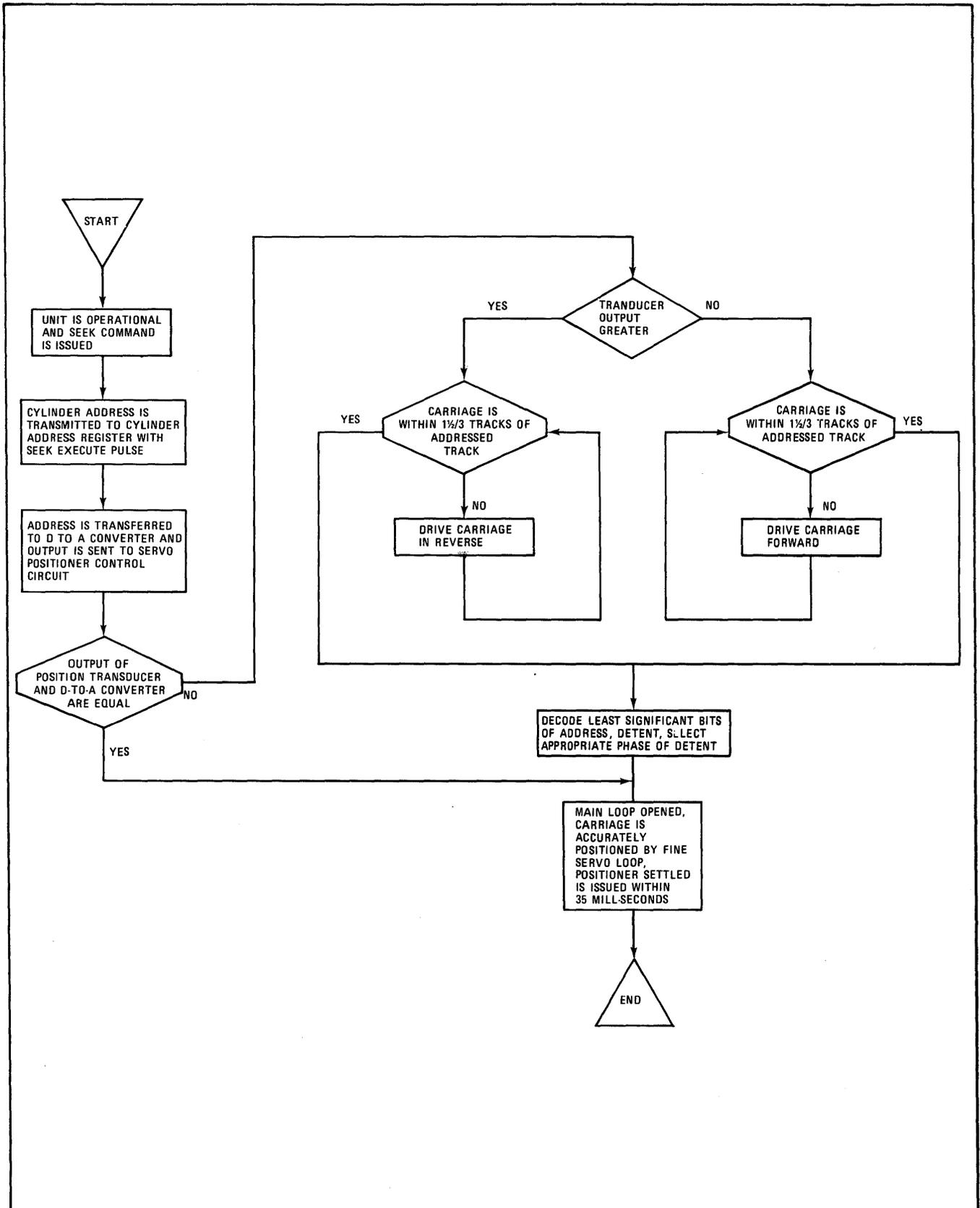
Figure 2-7. Operational Flow Chart Programmed Seek
