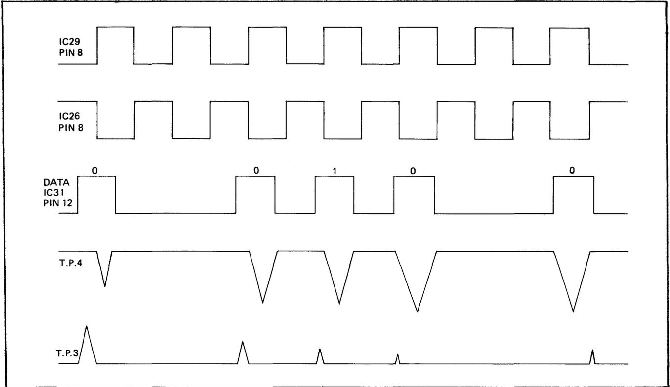
Figure 2-24. Phase-Locked Loop Timing Chart Data Frequency Too Low (Disk Rotating Slower)
