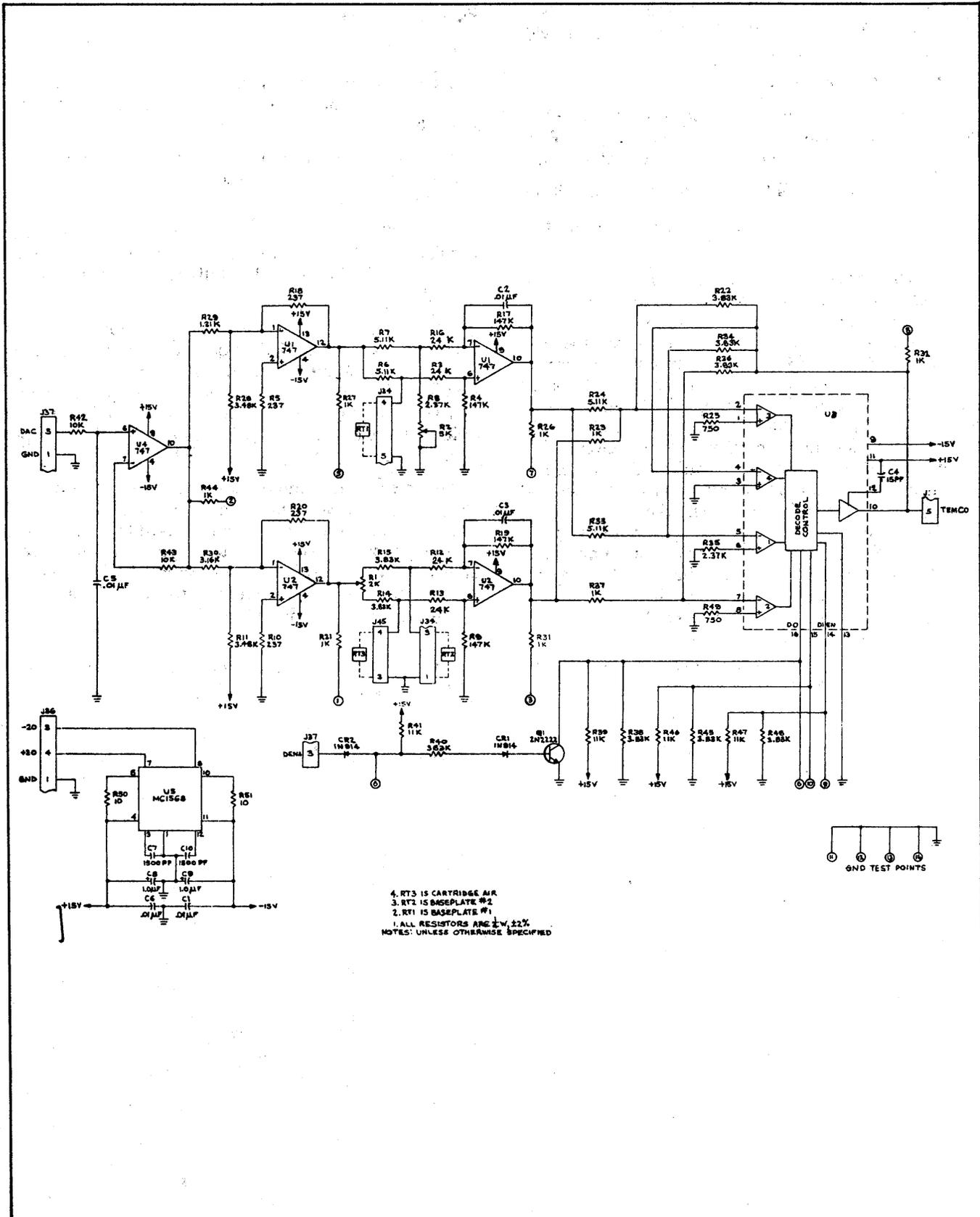
Figure 2-29. Temperature Compensation Board (9481-12 only)
