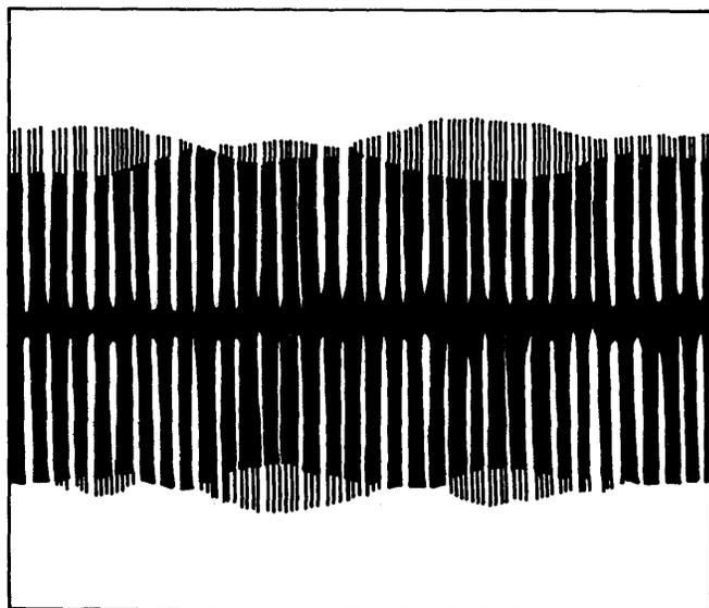
Figure 4-26b. DIBIT Patterns - Head Alignment - Correct
