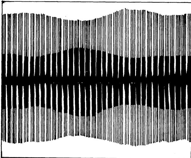
Figure 4-11a. Dibit Pattern-Head Alignment-Incorrect
