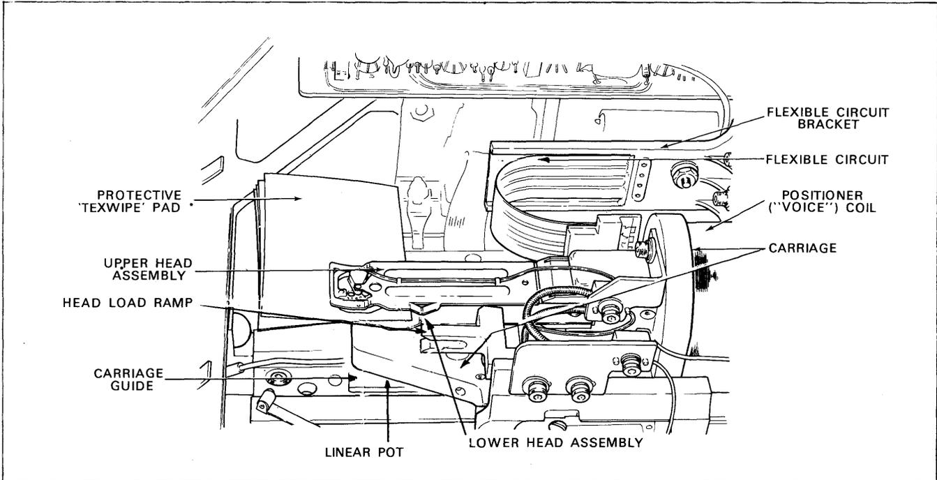
Figure 1-18. Positioner Mechanism (with protective pad in place between heads)
