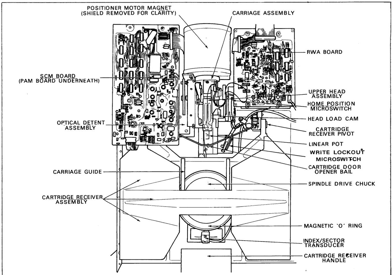
Figure 1-9. Plan View of 9480-12 Drive Module
