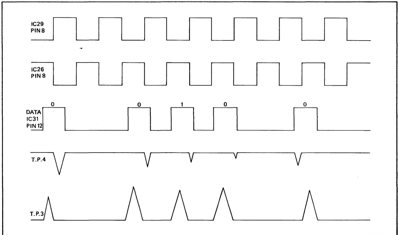
Figure 2-25. Phase-Locked Loop Timing Chart Data Frequency Too High (Disk Rotating Faster)
