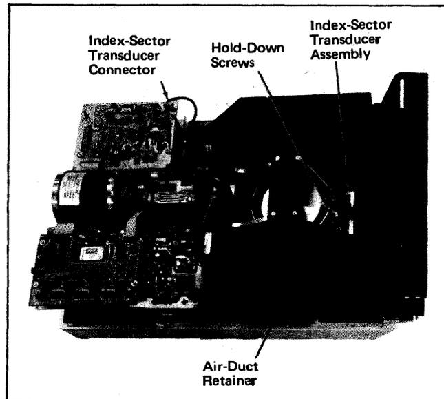
Figure 5-17. Index/Sector Transducer Assembly
