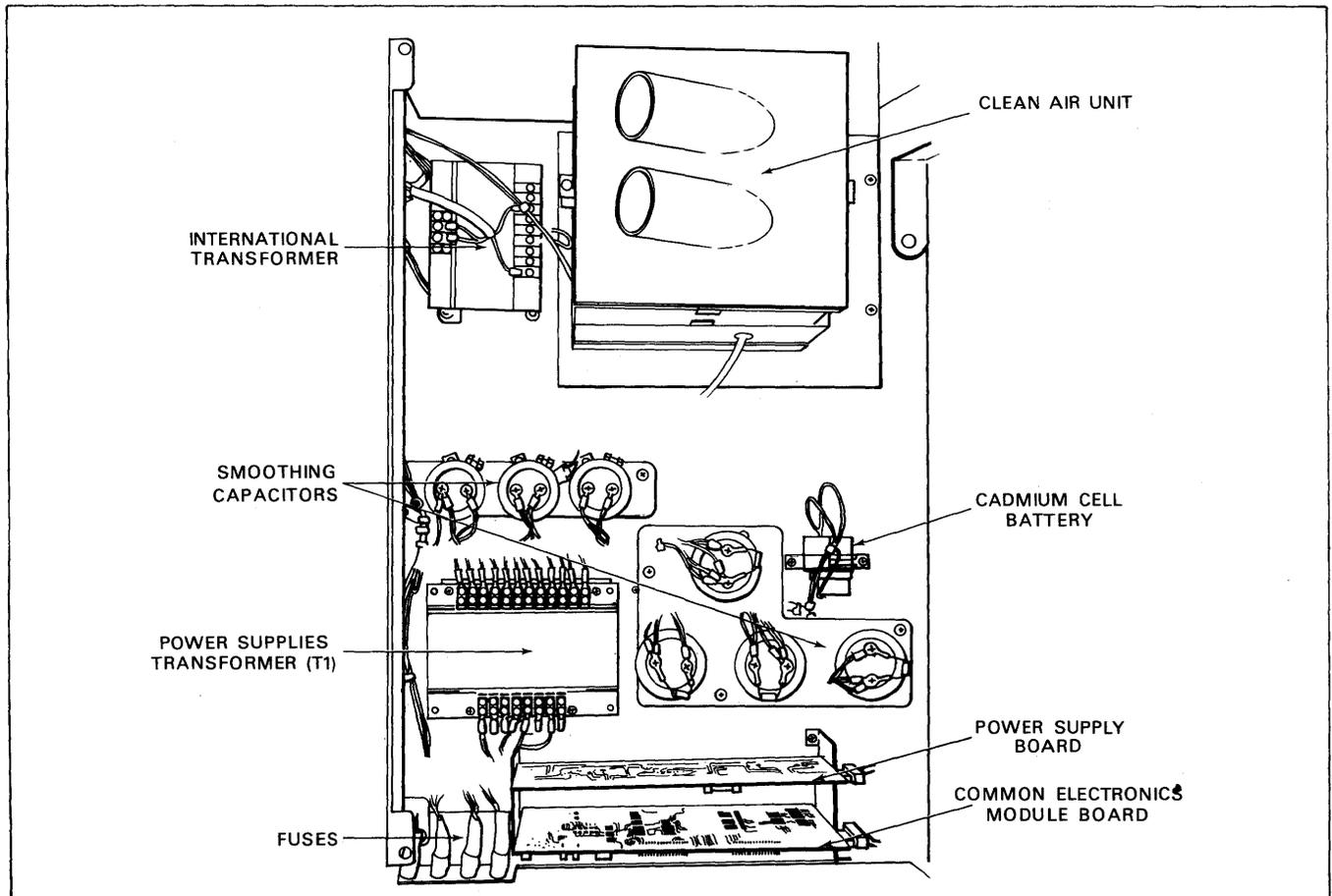
Figure 1-3. Plan View of Power Supply Area
