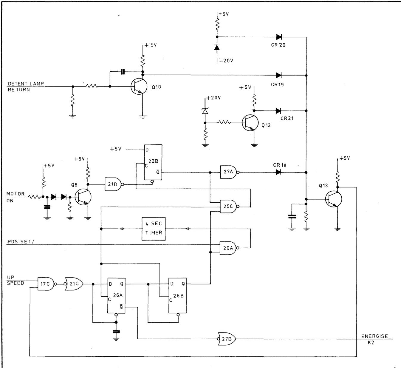
Figure 2-15. Failure Detection Circuitry.
