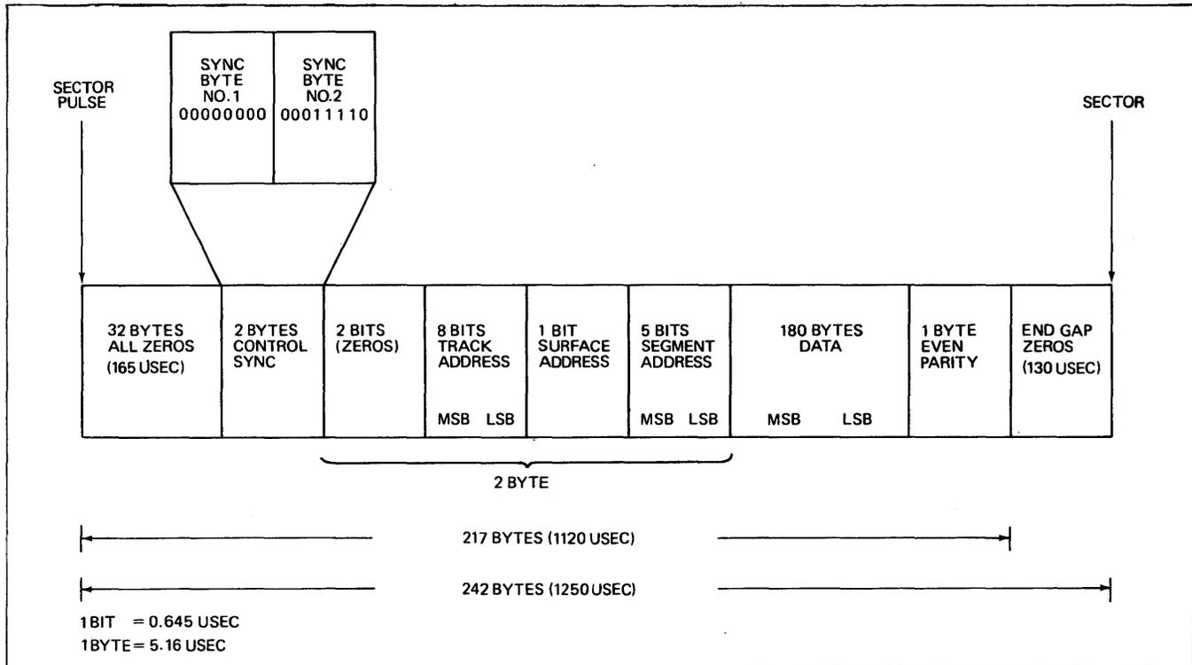
Figure 1-15. Burroughs DCD 2200 BPI 180 Byte Format
