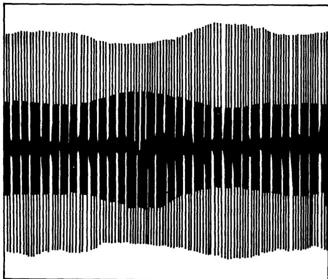
Figure 4-26a. DIBIT Patterns - Head Alignment - Incorrect
