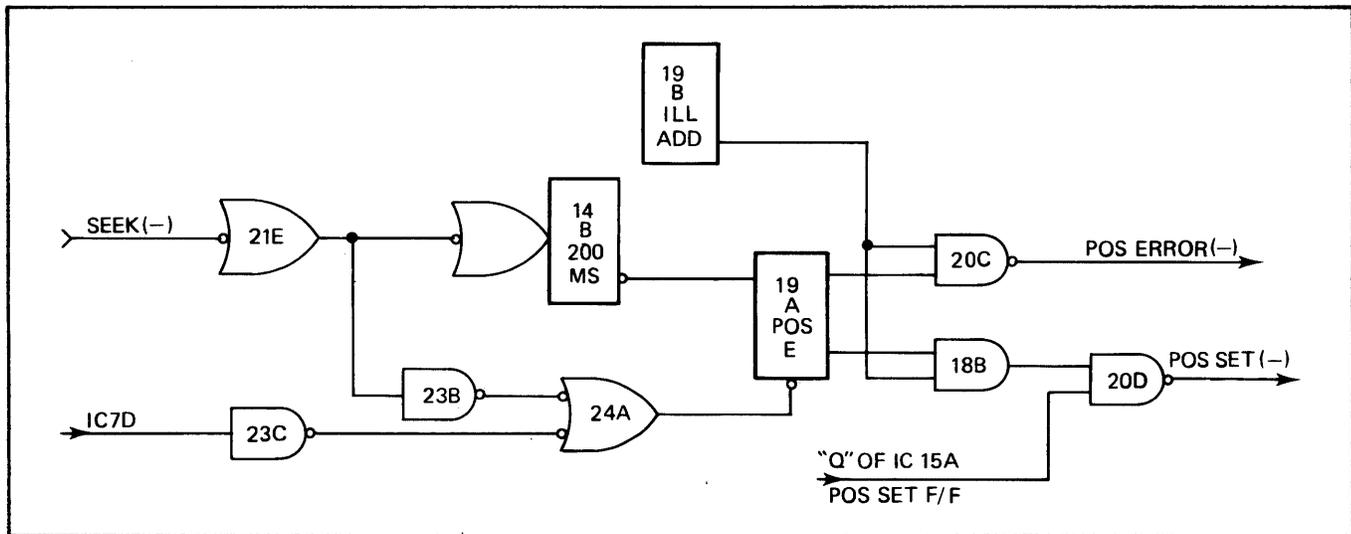
Figure 2-16. Position Error Detection.
