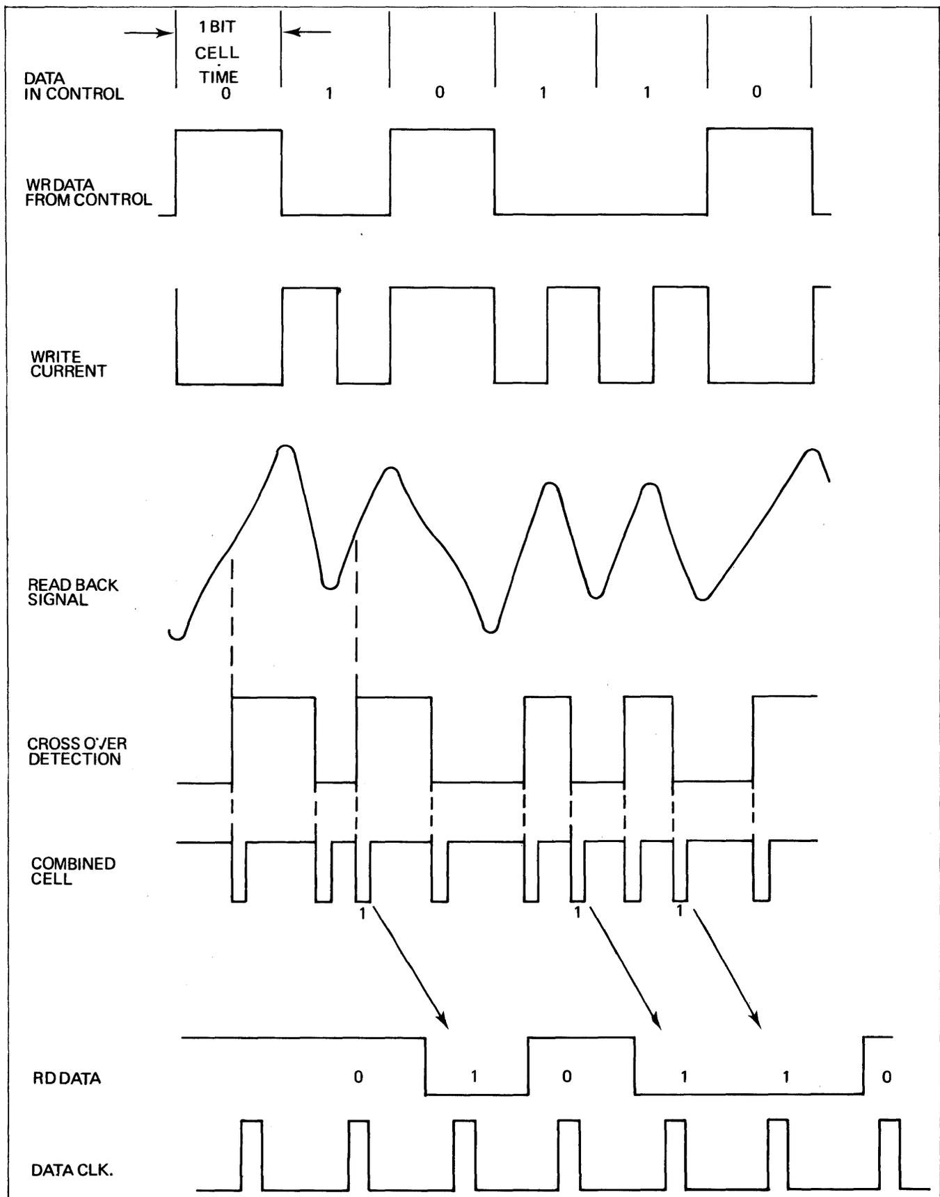
Figure 1-14. Double Frequency Recording
