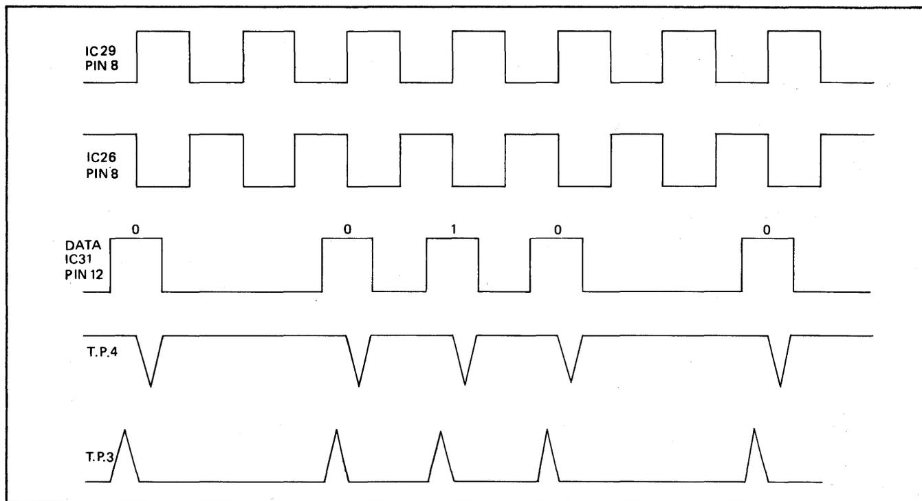
Figure 2-23. Phase-Locked Loop Timing Chart Data And Clocks Synchronized
