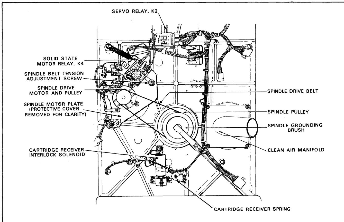
Figure 5-19. Spindle Drive Motor Assembly
