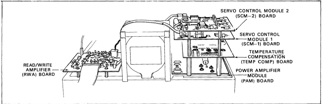
Figure 1-25. Rear View of Module Showing Boards (9481-12)
