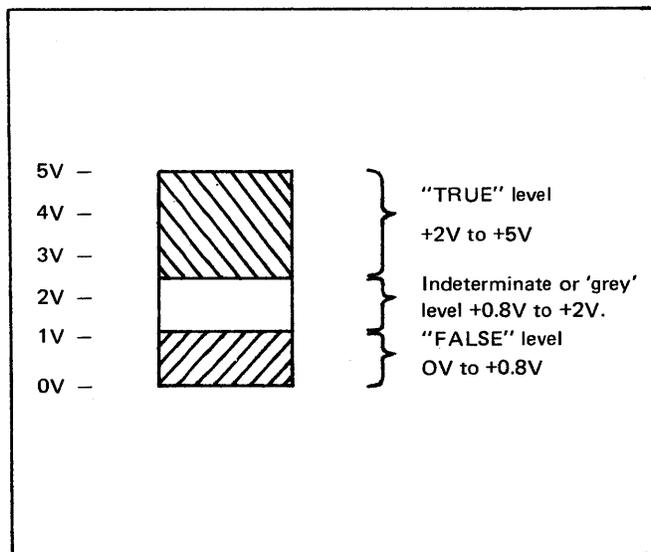
In general, a TRUE is considered as "HIGH" and FALSE is considered "LOW", but there are some exceptions on interface lines and inter-board signals. A PLUS (+) or MINUS (-) sign next to a signal name indicates the active state of the signal, for example:
