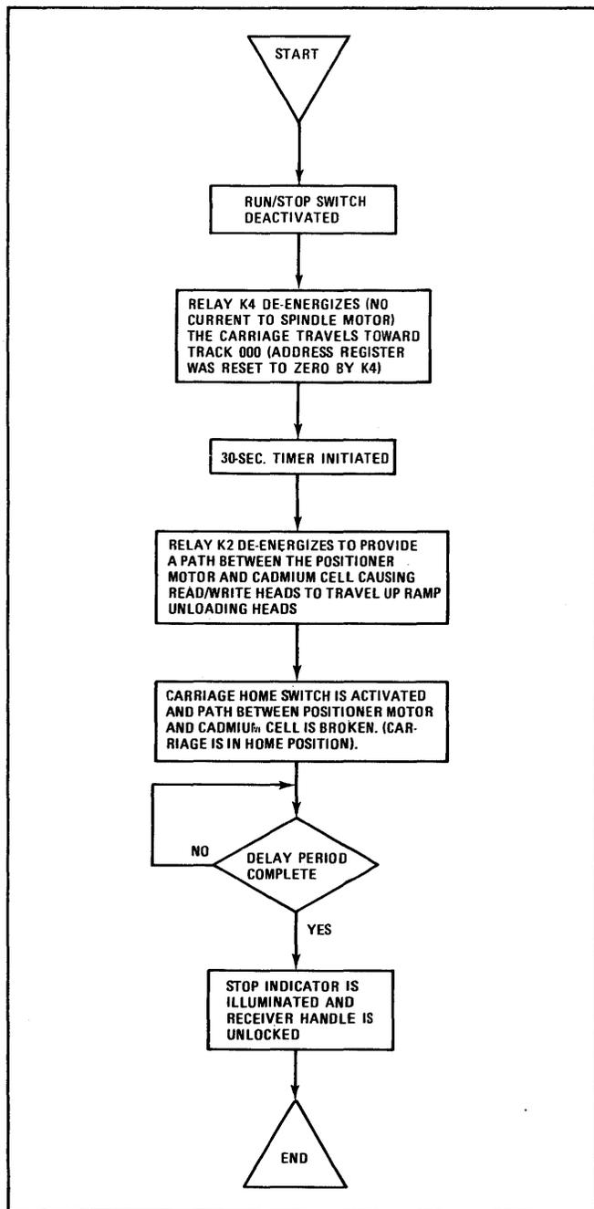
Figure 2-6. Power-Down And Head Retraction Flow Chart
