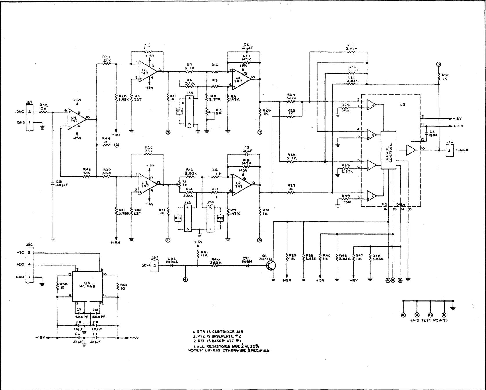
Figure 3-16. 9481-12 Temperature Compensation Board
