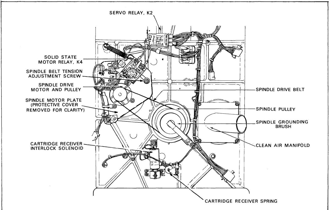
Figure 1-11. Bottom View of Drive Module
