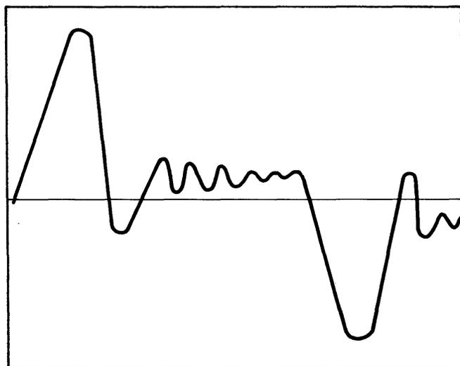
Figure 4-25a. Servo Offset Adjustment - Incorrect
