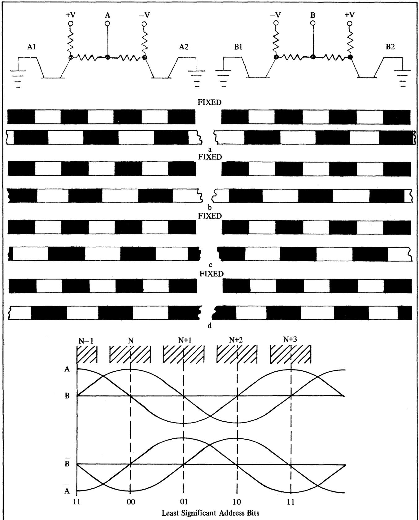
Figure 2-11. 9480-12 Optical Detent
