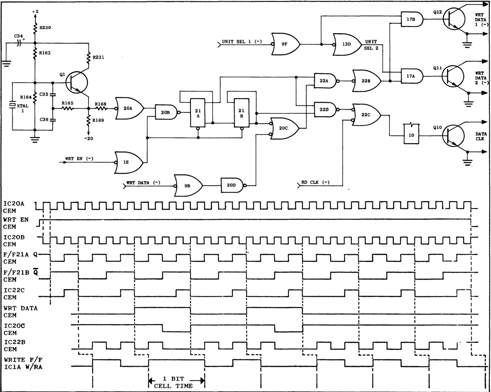
Figure 2-18. Write Data Encoder Part of CEM
