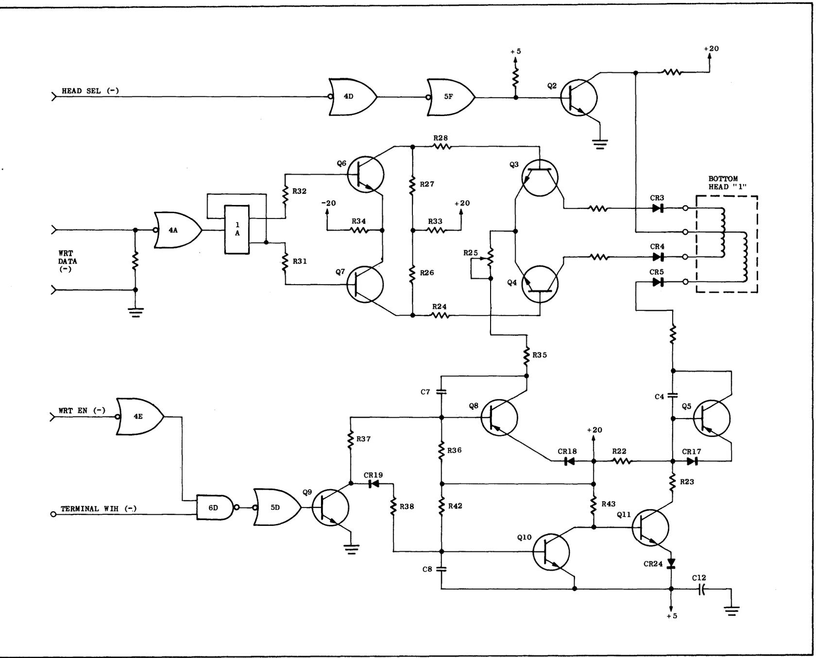
Figure 2-19. Write Amplifiers and Drivers.
