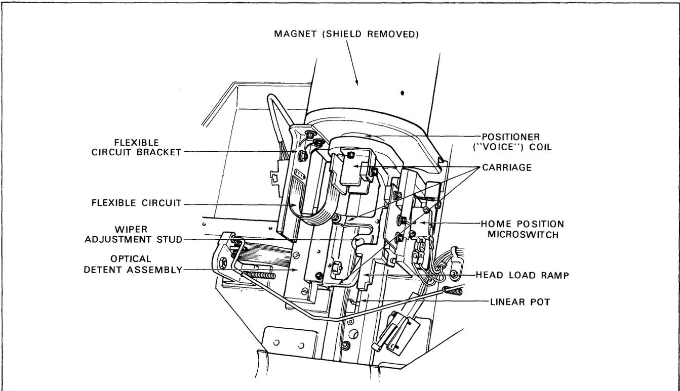
Figure 1-19. Positioning System Components (Heads and Boards Removed for Clarity)
