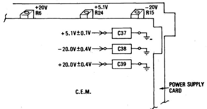
Figure 6-9. Voltage Adjustments
