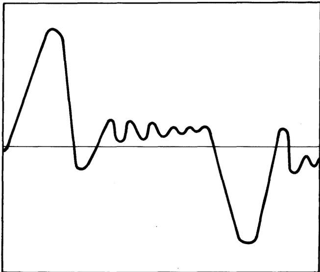
Figure 4-10a. Servo Offset Adjustment – Incorrect
