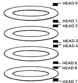
**Figure 1-5. Platter Configuration (207)**
