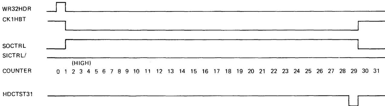
Figure 3-9. Header Control Write Header
