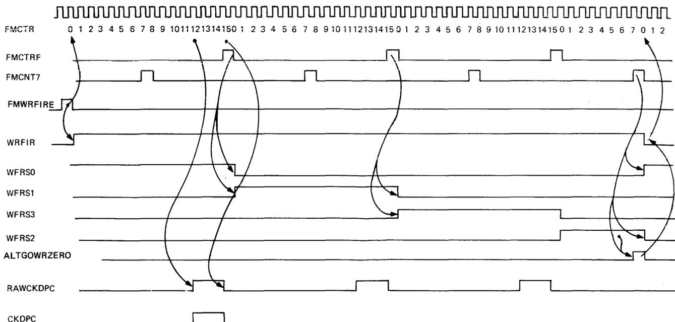
Figure 4-10. WRITE FIRE State Logic (207)
