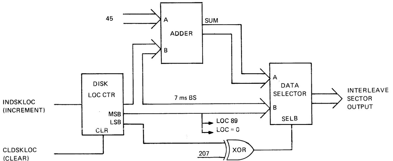
Figure 3-1. Disk Location Counter and Interleave Logic
