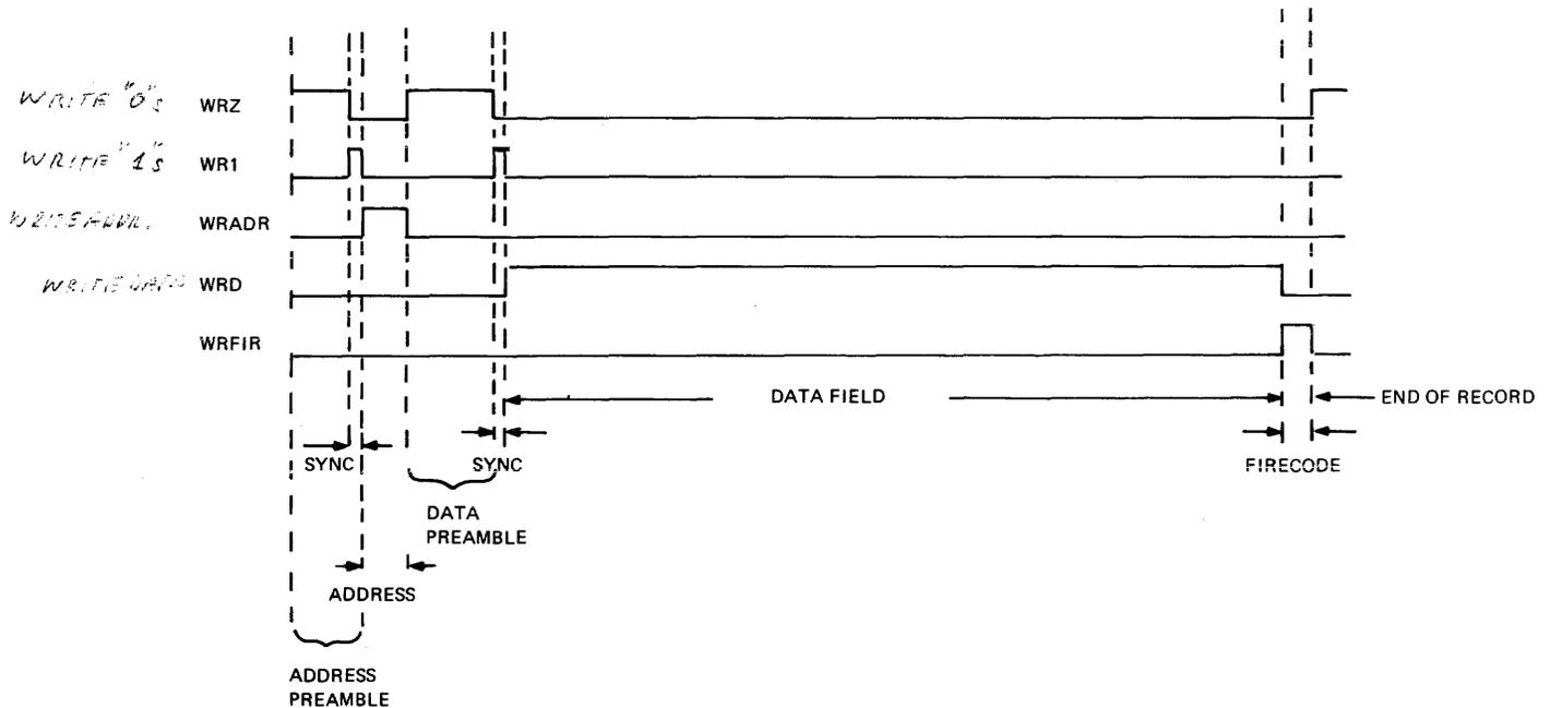
Figure 4-5. Format Signals During Initialize of One Sector
