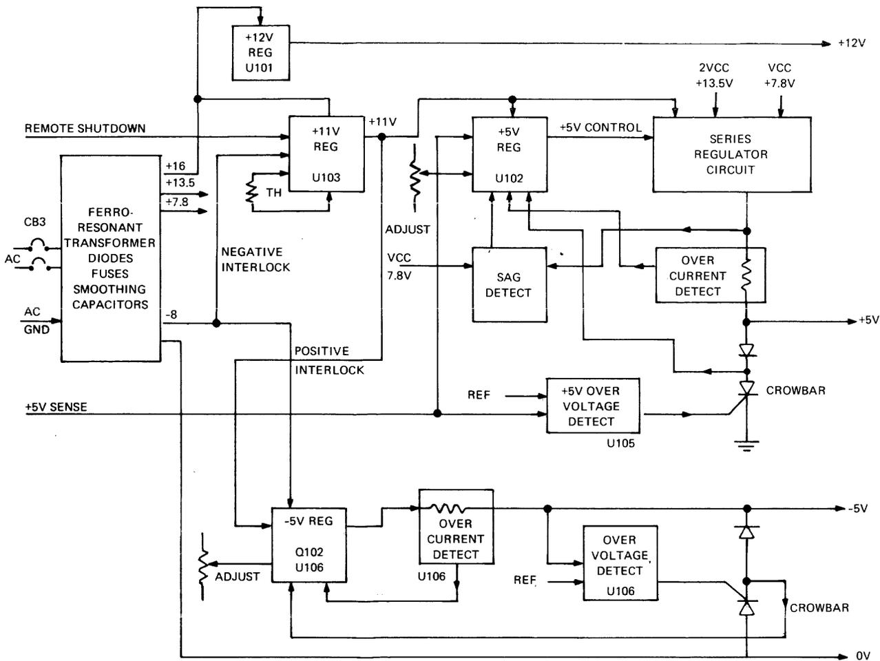
Figure 6-1. Power Supply Block Diagram
