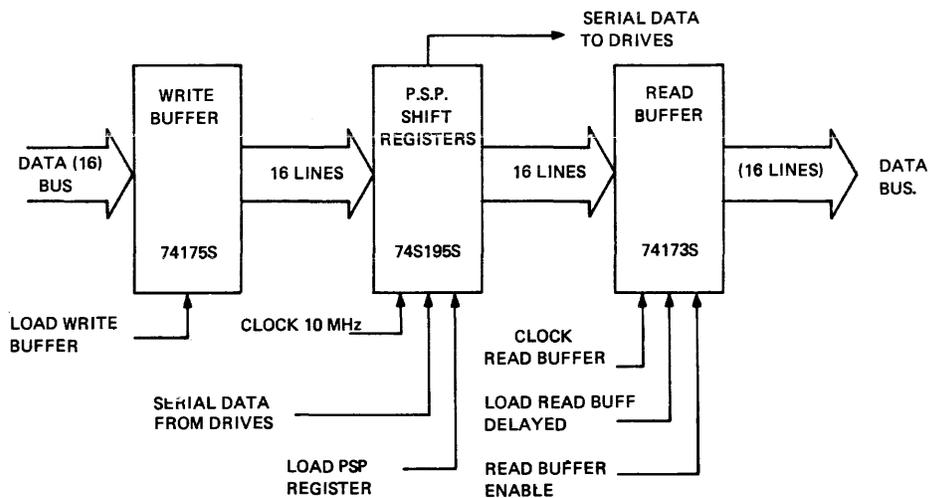
Figure 4-13. Parallel/Serial/Parallel Register
