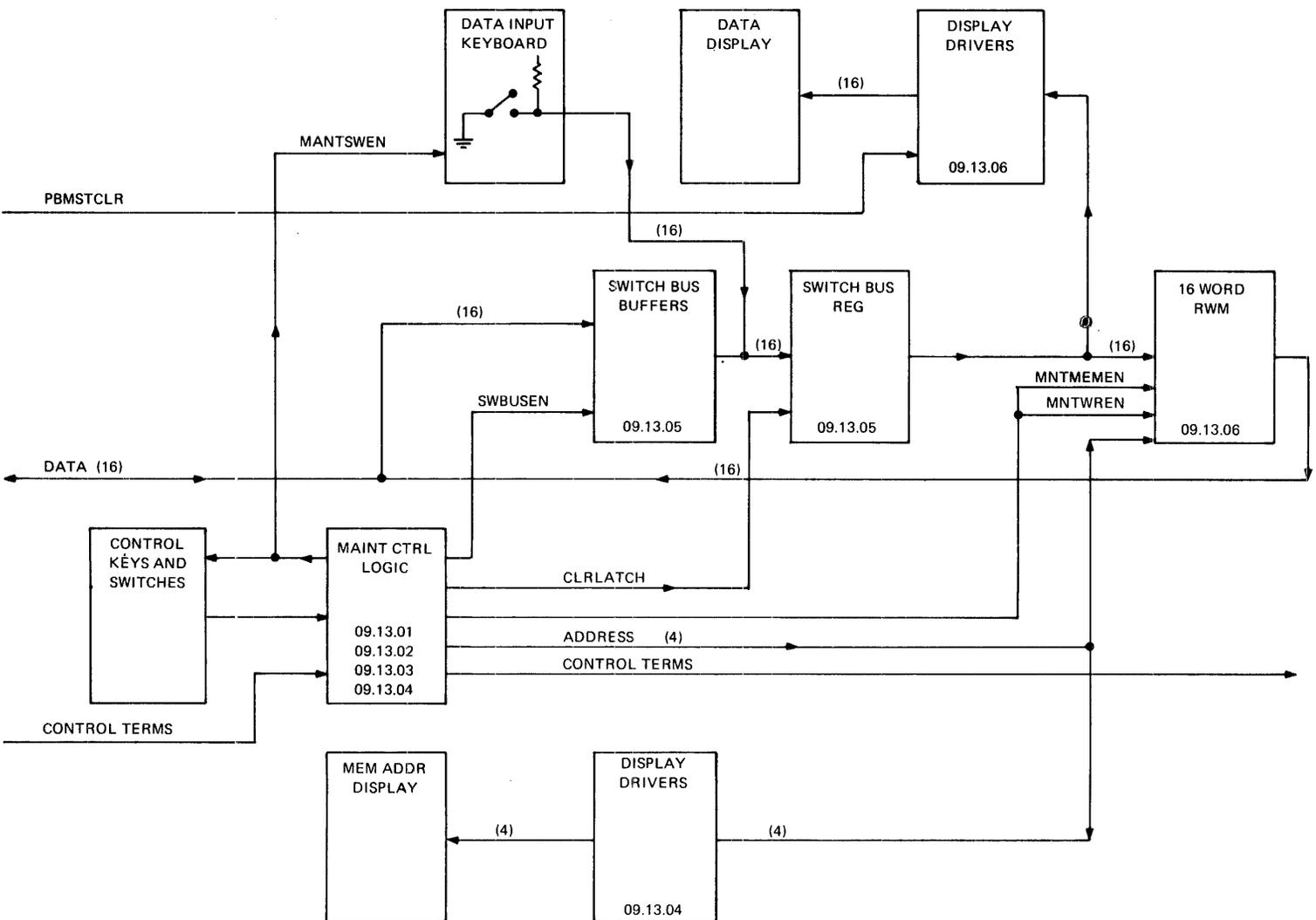
Figure 5-15. Maintenance Logic
