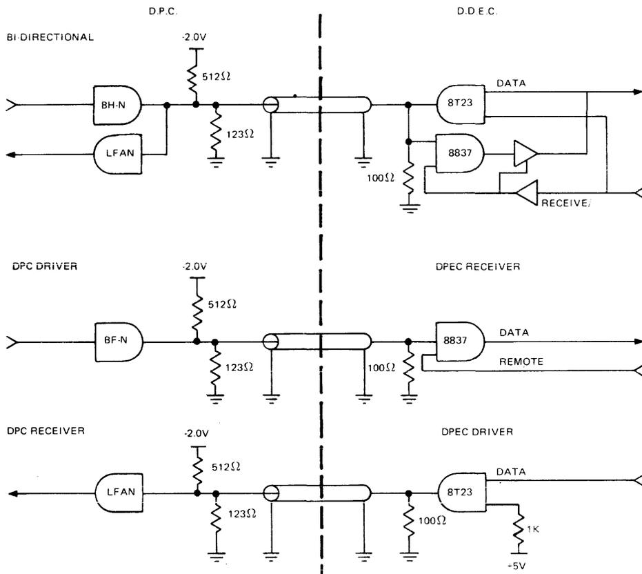
Figure 1-8. Interface Connections
