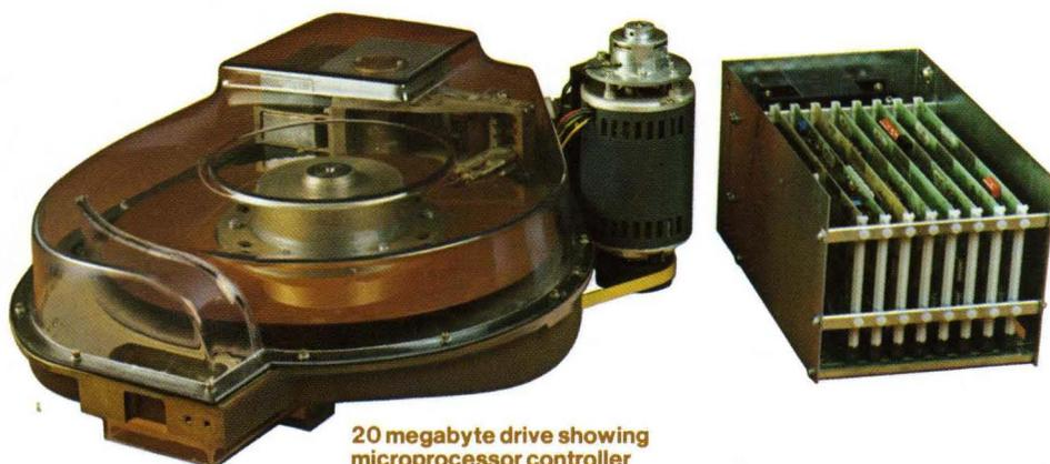
20 megabyte drive showing microprocessor controller (right).
