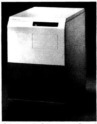
The Unisys A1, A4, and A6 systems consist of a central processor, 12 megabytes of main memory, I/O and data communications subsystems, and a maintenance subsystem. All these components are contained in a cabinet with a footprint of only 3.67 square feet.
