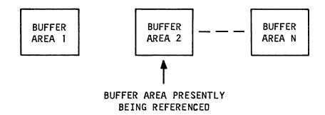
If the file pertains to input information, then buffer area 1 is refilled with the next record. If the file pertains to output information, then information from buffer area 1 is transferred to the appropriate output unit.
