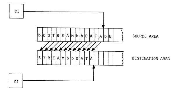
3-34. TRANSFER AND CONVERT OPERATION. There are two forms of the \( \tansfer type \) s for transfer and convert operations. These two forms have been specified to handle both input and output conversions.
