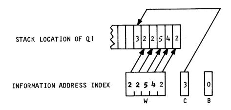
3-19. The last form of the (store address statement) provides the programmer with the ability to store the setting of the control index. This form of the (store address statement) has the following format:
