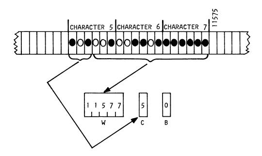
3-17. STORE ADDRESS STATEMENT. There are three forms of the (store address statement). The first two forms enable the programmer to store the settings of the source or destination indexes. The third form is used to store the setting of the control index. The first two forms have the following format:
