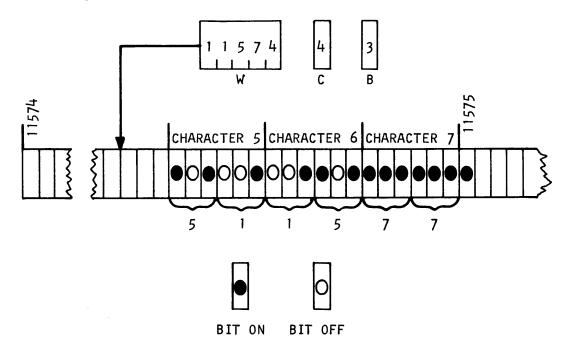
pointer is adjusted to zero and the character pointer is counted up one, if necessary ( $SI_b \neq 0$ ). The address index, SI in this case, is set to the value of the next 18 bits of the string. The first three bits set the character portion of the index, and the next 15 bits set the word portion of the index. The bit portion of the index is set to zero.
