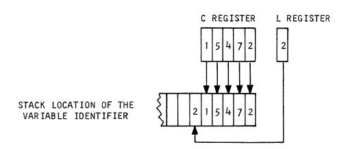
3-21. RECALL ADDRESS STATEMENT. The (recall address statement) has three forms which are the counterparts of the (store address statement). The first two forms allow the programmer to set the source or destination indexes to the location of some variable. The third form is used to recall a previous setting of the control index. The first two forms have the following formats:
