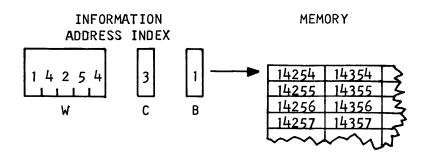
and the statement DI  $\leftarrow$  Q1 is executed. The address index, DI in this case, is set to the value of Q1. The word portion of the index is set to the value of the 15 low-order bits. The character portion of the index is set with the next three high-order bits.
