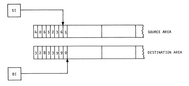
3-50. TRANSFER CHARACTER PORTION. This transfer type has two forms. The first form transfers the zone bits from the source string to the destination string. The second form transfers the numeric bits from the source string to the destination string. Each of these forms is discussed in detail below.
