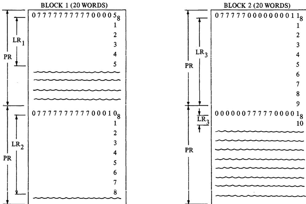
Note that the control word uses one word of the physical record, and that the ten word logical record (1,2,..., 10) could not be completely contained in the first physical record of block two.
