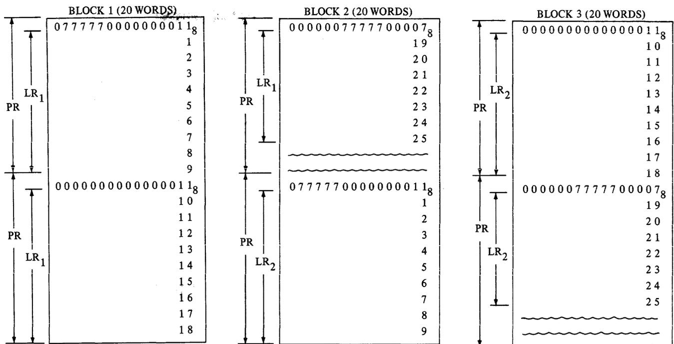
If the logical record is greater than or equal to the physical record, then the first (PR-1) words of the logical record will be contained in the first associated physical record.
