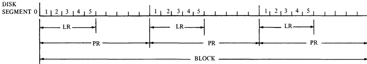
For maximum efficiency let PR=5, and the BLOCKING factor=6. The substitution of these values will create six 5-word logical records on one disk segment.
