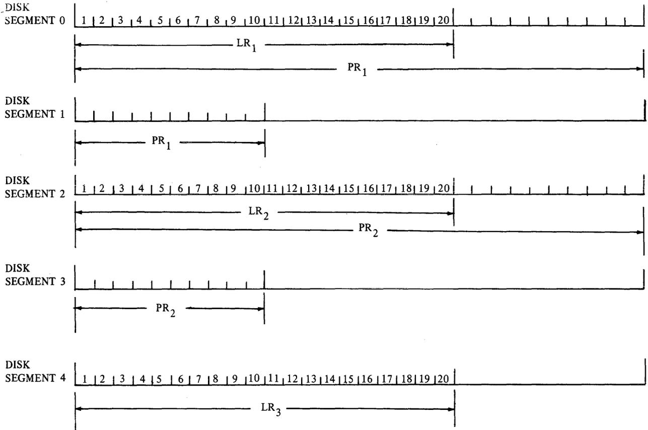
Since the blocking factor is undeclared, the physical record size also becomes the block size. In the above example, each block requires two disk segments.
