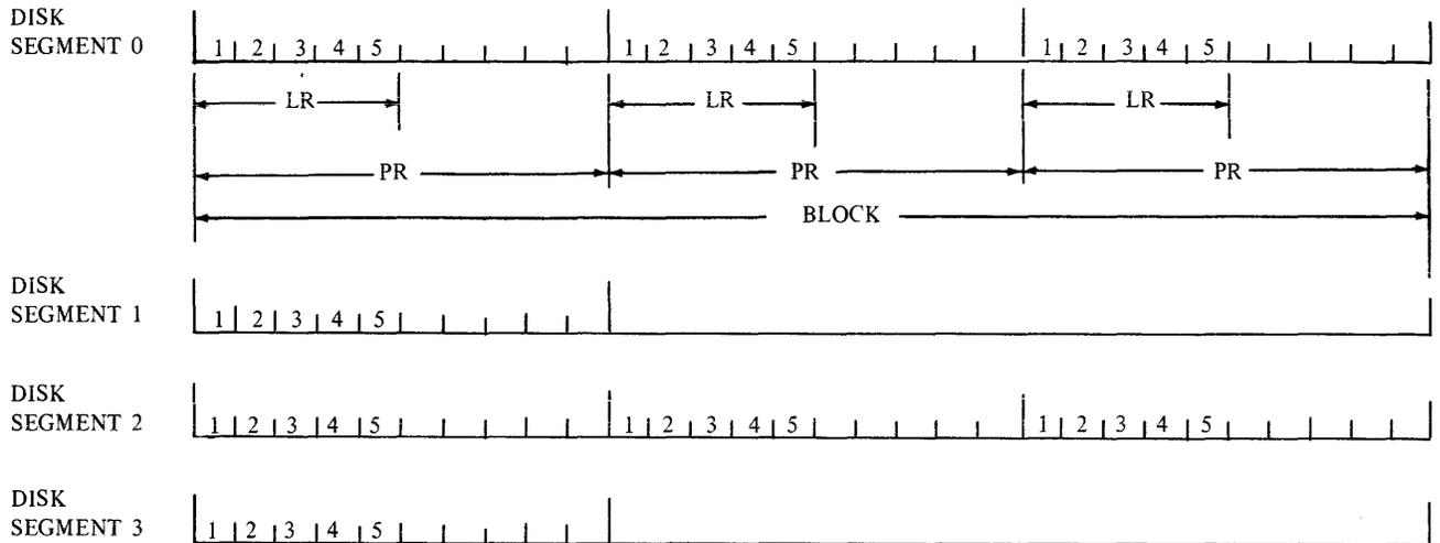
If a blocking factor of six had been specified, six records could be contained in two disk segments.
