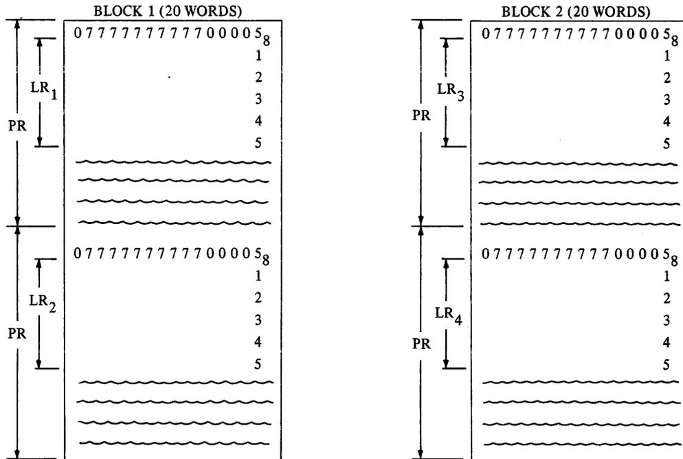
The block size of a tape file is determined by multiplying the BLOCKING factor by the physical record length. The block size in example 1 is 2 x 10 = 20 words.
