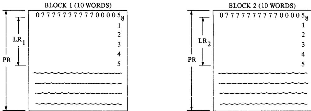
An unblocked tape file implies, and is implied by a blocking factor of one.
