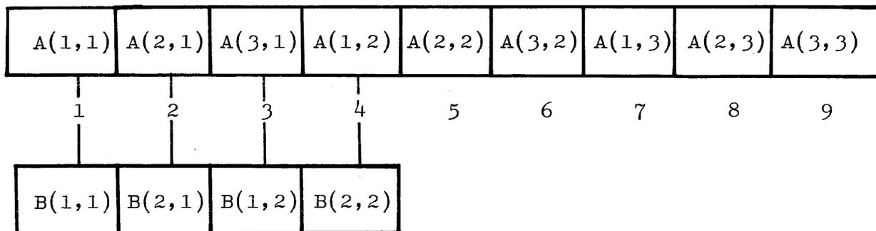
The mapping is always set-up so that the n elements of the subroutine array will correspond to the first n elements of the array passed to it in the calling program.
