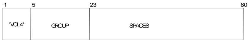
**Figure E-19. ANSI87 Volume Header 4-Non-Scratch**
