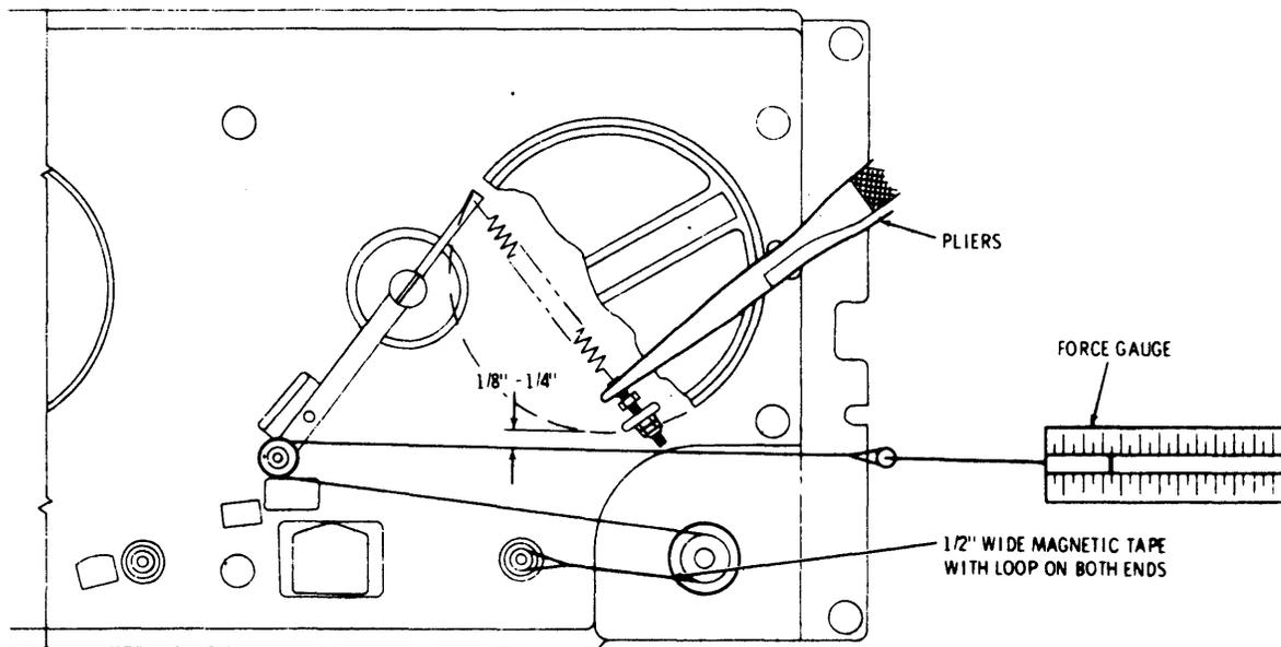
Figure 6-8. Tension Adjustment for Take-up Reel
