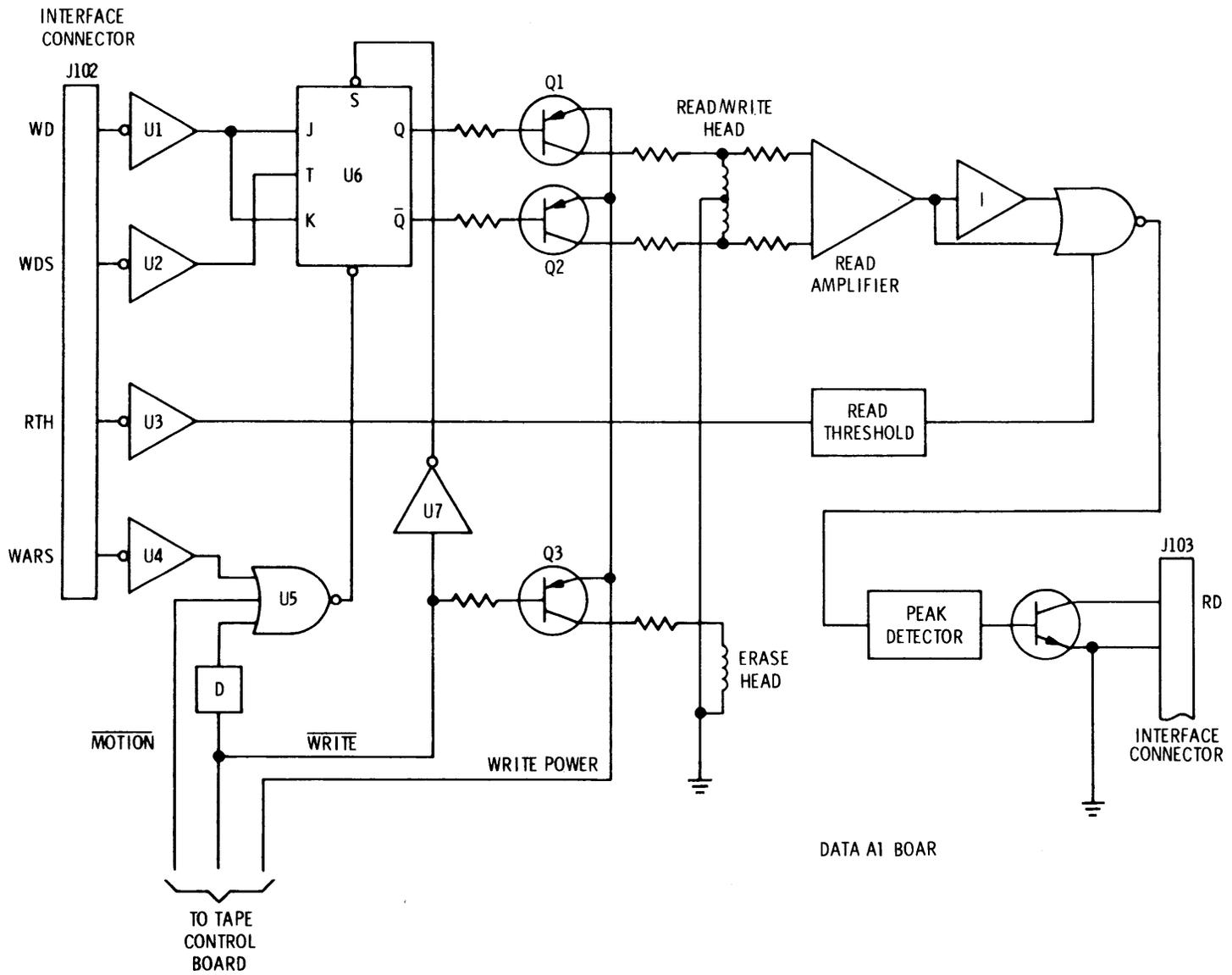
Figure 4-10. One Channel of Data Electronics
