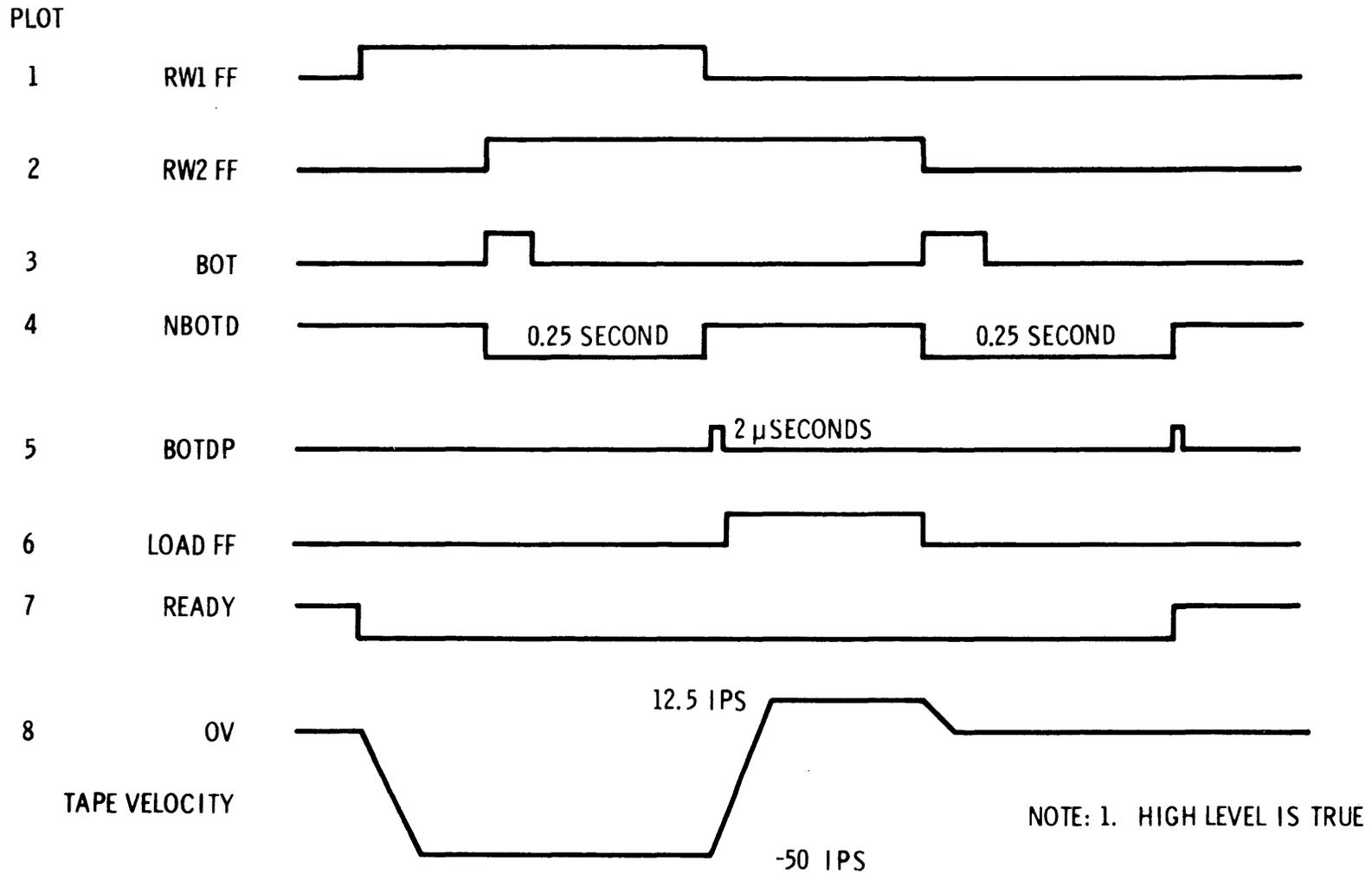
Figure 4-17. Tape Control Waveforms During Rewind to Load Point Sequence
