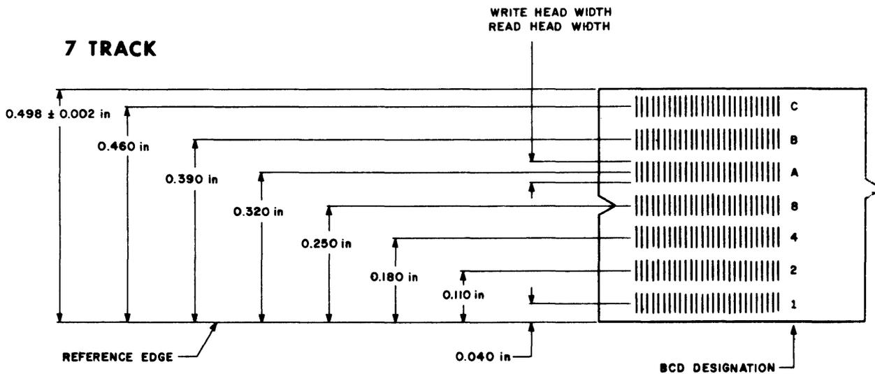
Figure 4-8. 7-Track Allocation and Spacing
