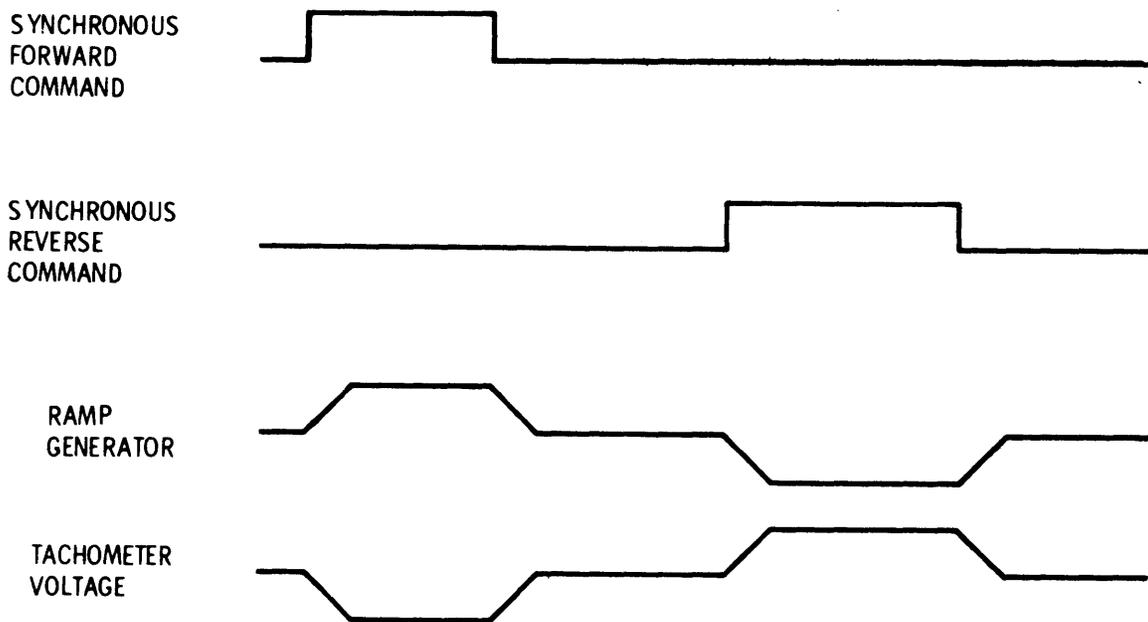
Figure 4-5. Typical Capstan Servo Waveforms
