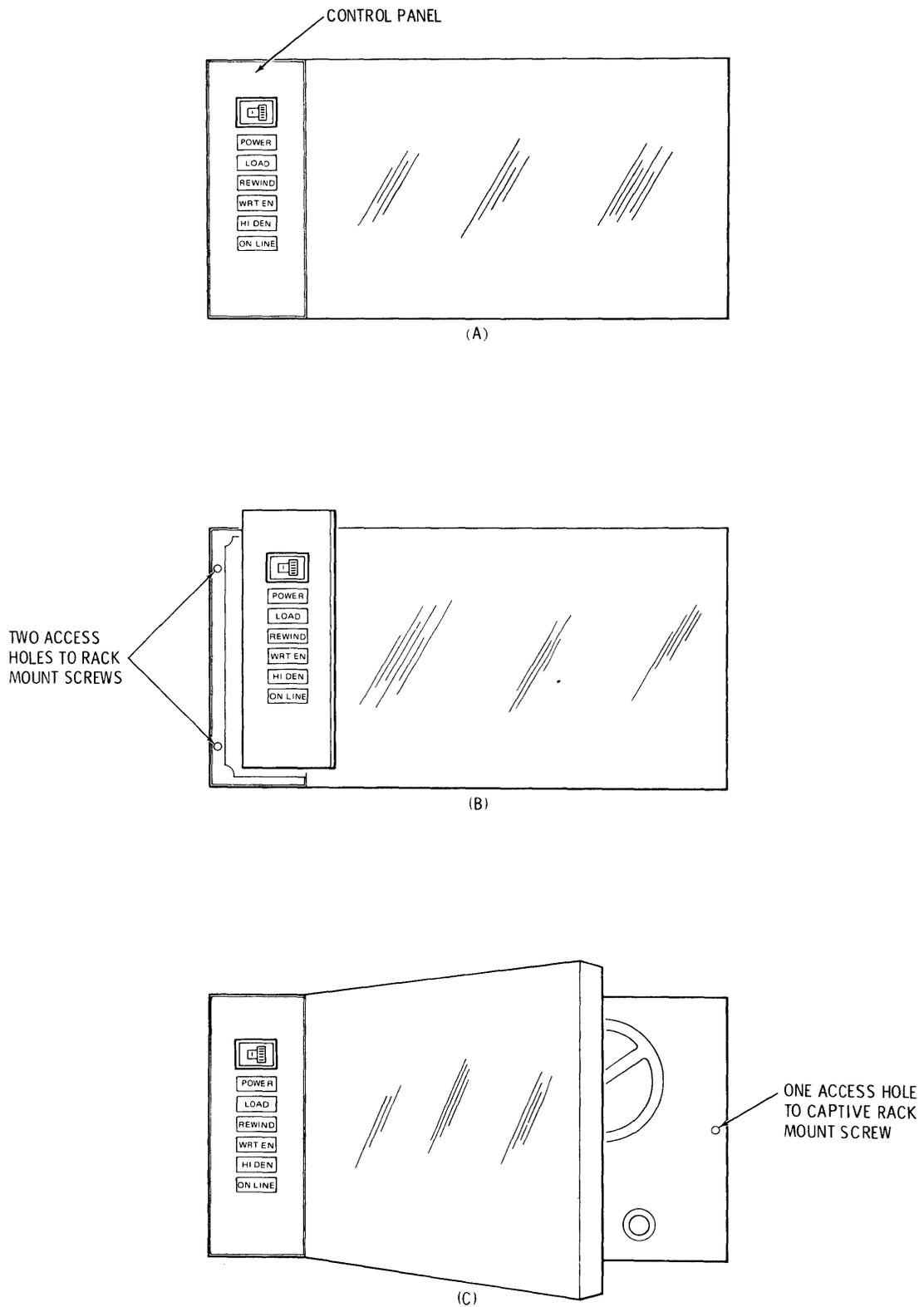
✓ Figure 2-2. Rack Mounting the Transport
