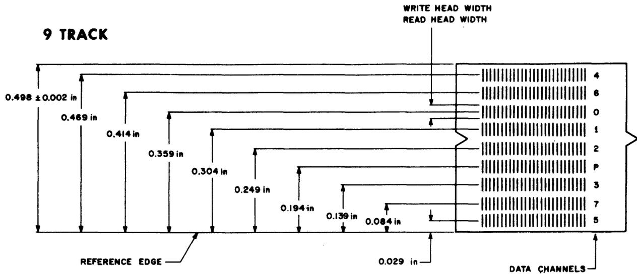
Figure 4-7. 9-Track Allocation and Spacing
