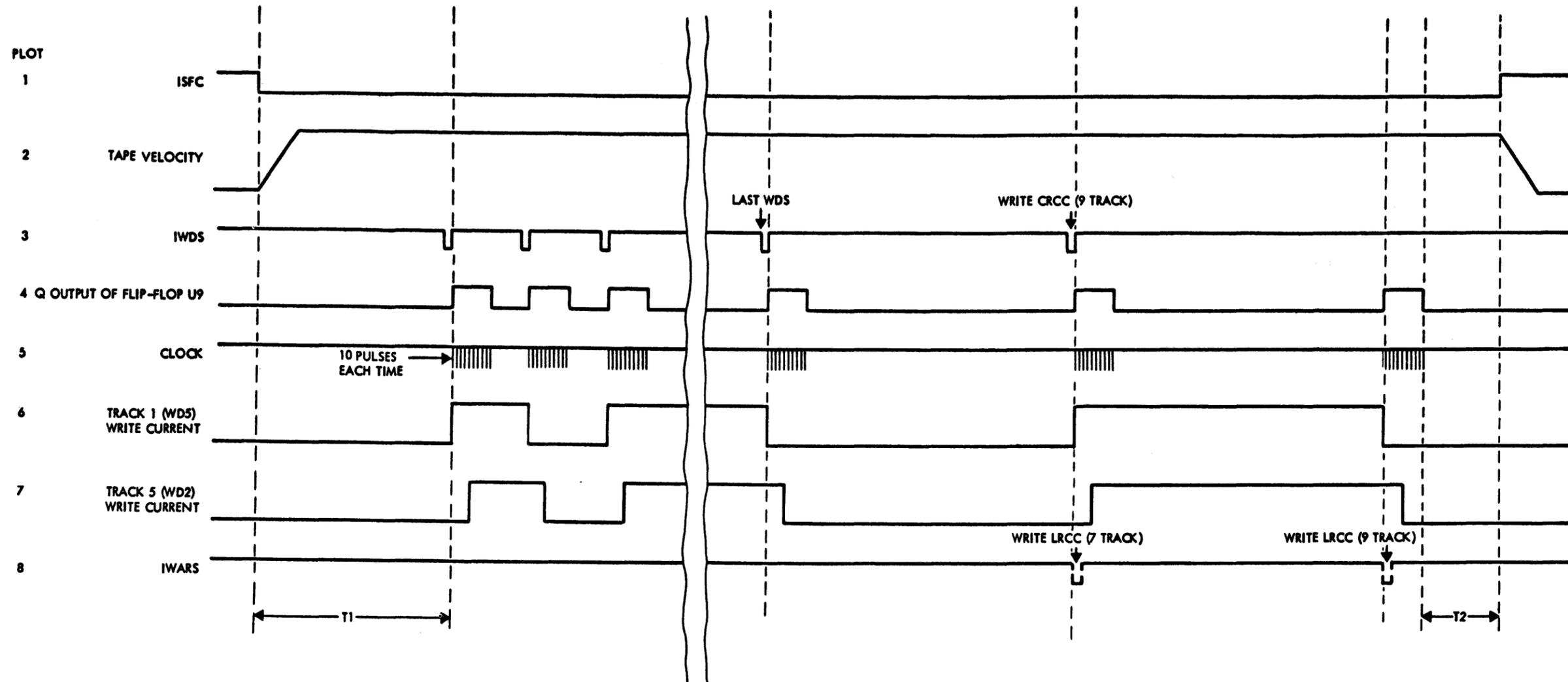
Figure 4-22 . Timing Diagram, Data Recording
