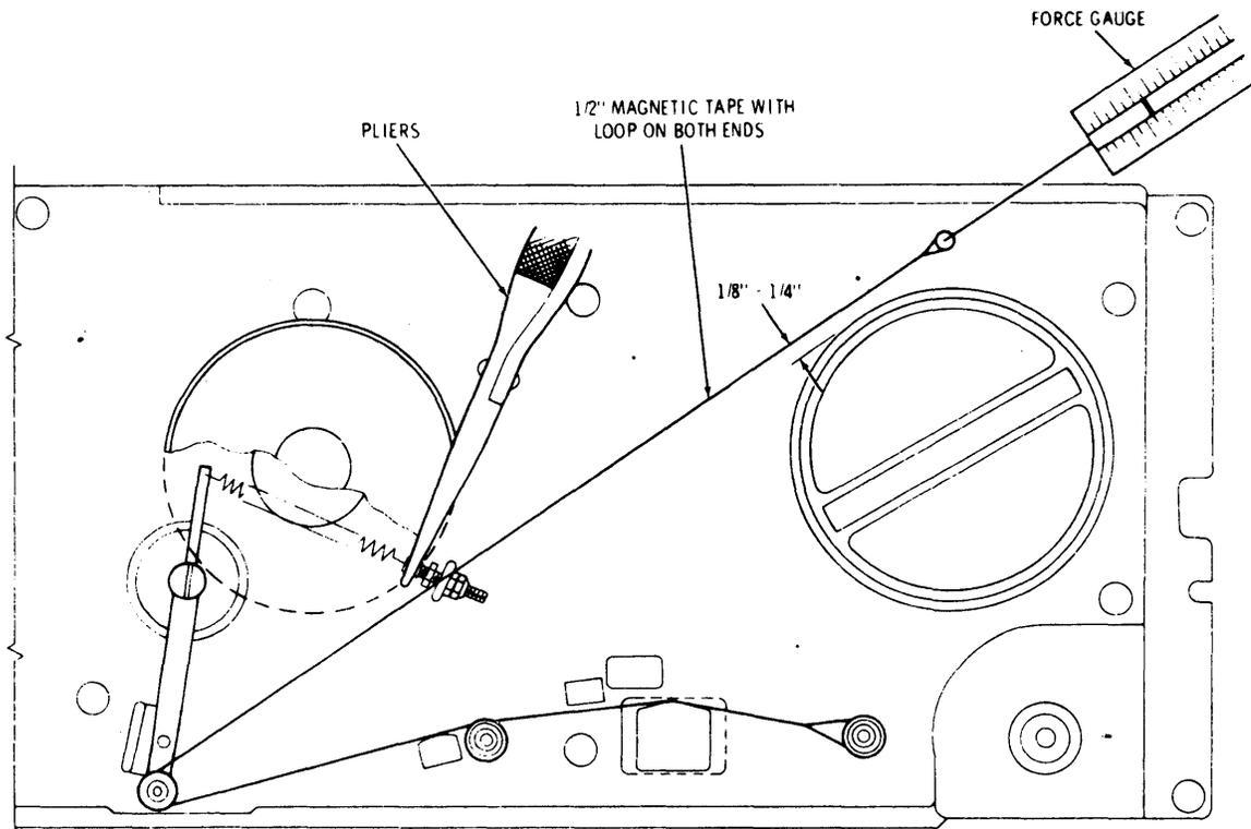
Figure 6-7. Tension Adjustment for Supply Reel
