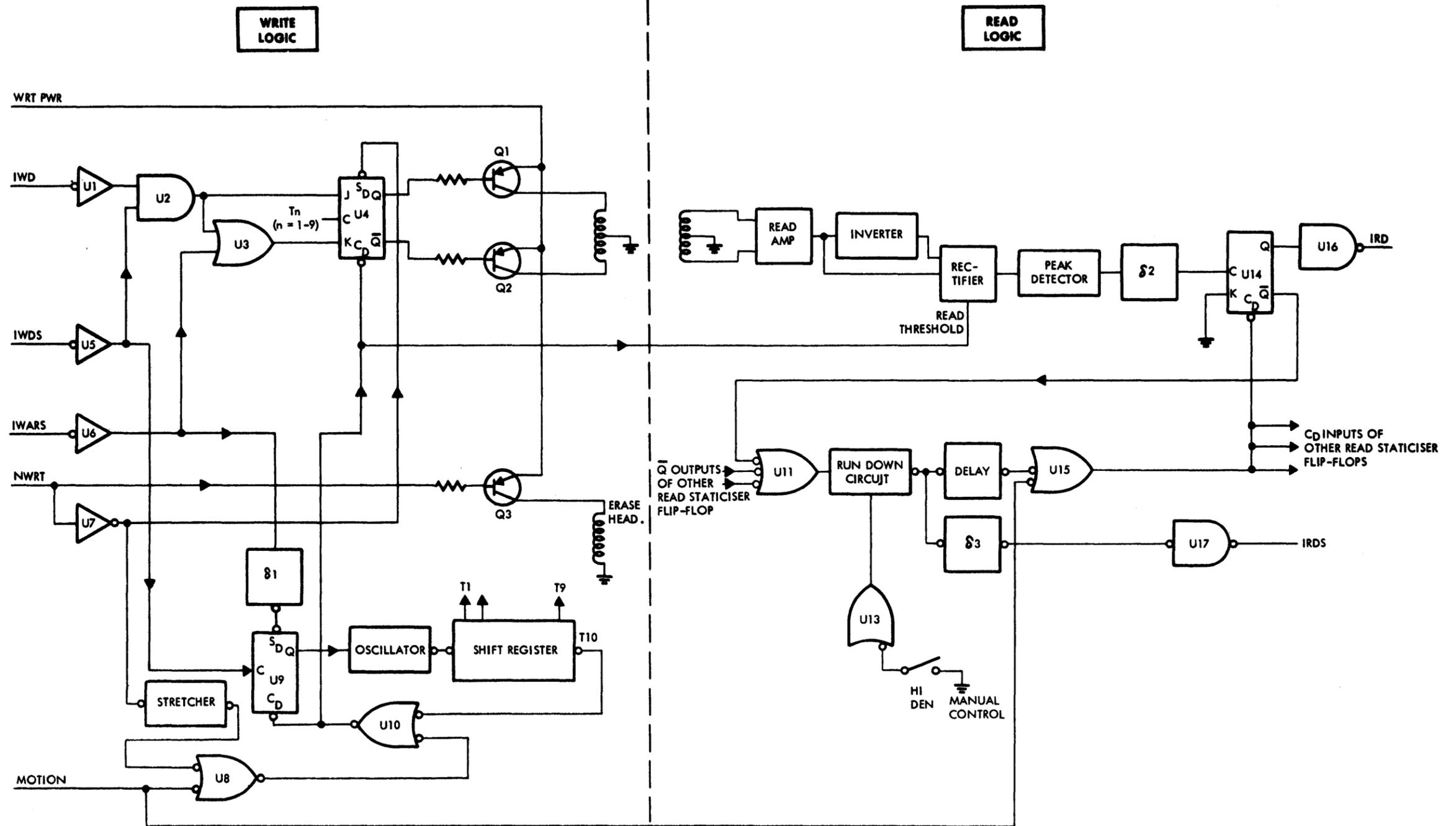
Figure 4-21 . Block Diagram, One Channel of Data Electronics
