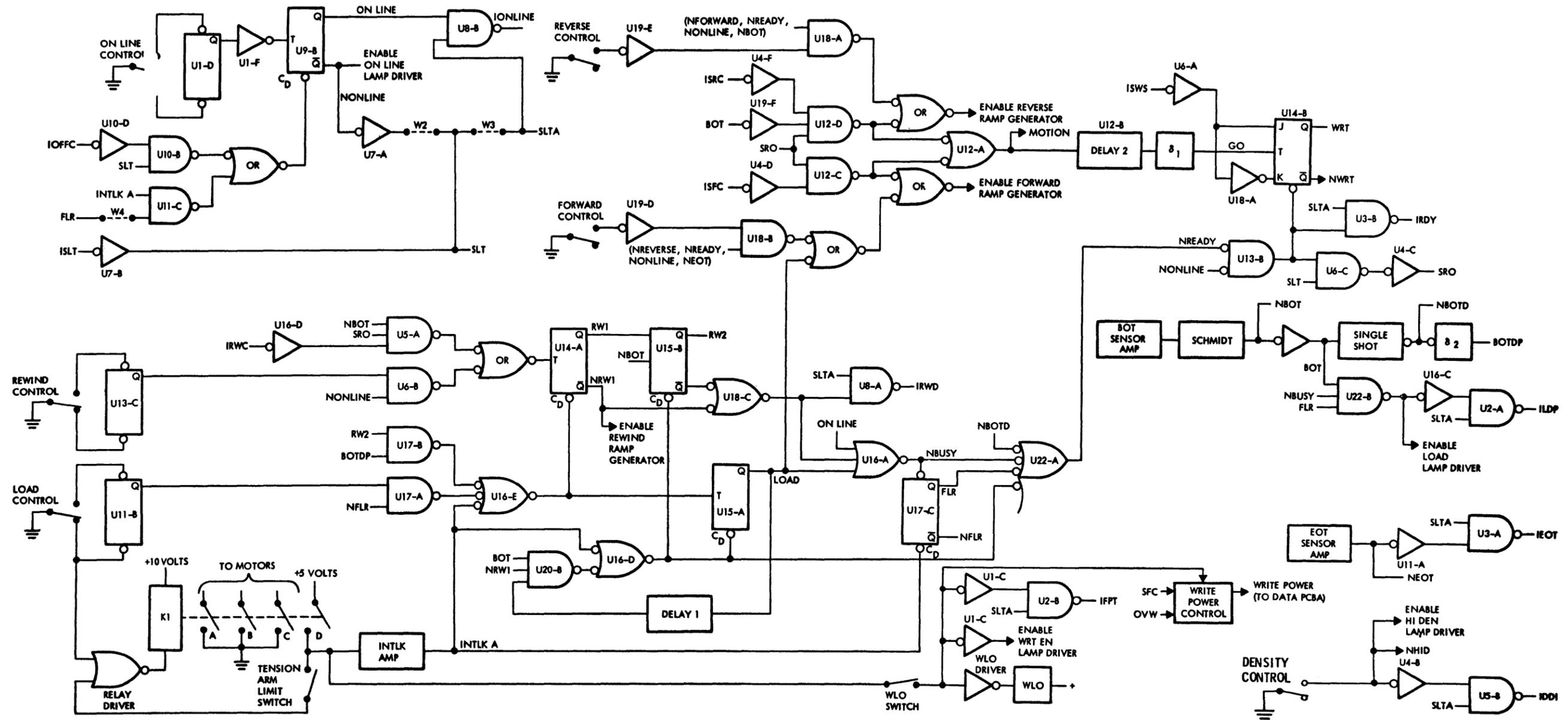
Figure 4-24, Block Diagram, Tape Control Logic
