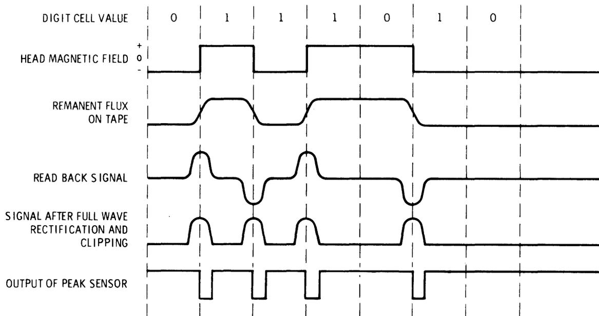
Figure 4-9. Write and Read Waveforms
