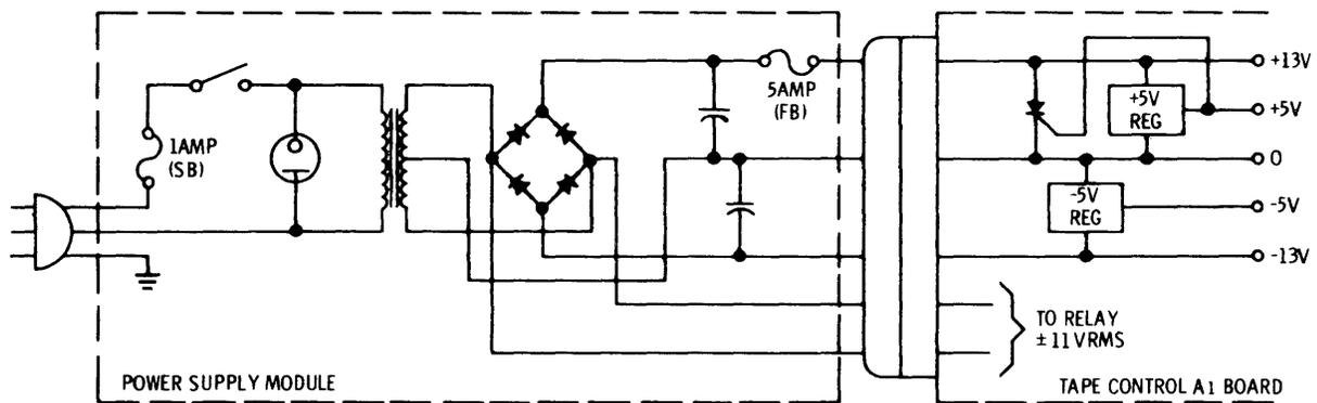
Figure 4-2. Block Diagram of Power Supplies
