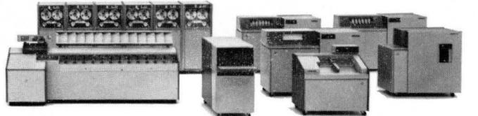
**B 260 PUNCHED CARD SYSTEM:** It combines collation, computation, summarization and hard-copy preparation all in one run. Completely buffered for maximum throughput. Highly automatic operation and scheduling.
