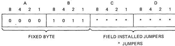
**Figure 4-36. Reader Sorter DLP Test/ID Word 2 Result Descriptor**
