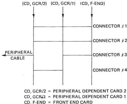
Figure 4-55. GCR Tape DLP Frontplane Connectors
