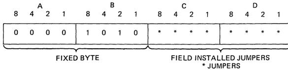
**Figure 4-23. 5N DF DLP Test/ID Word 2 Result Descriptor**
