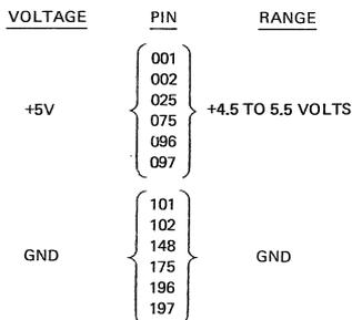
Figure 4-56. GCR Tape DLP Voltage Test Points
