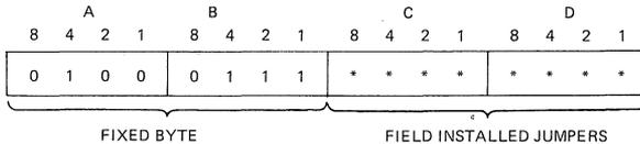
Figure 4-49. Uniline DLP Test/ID Result Descriptor
