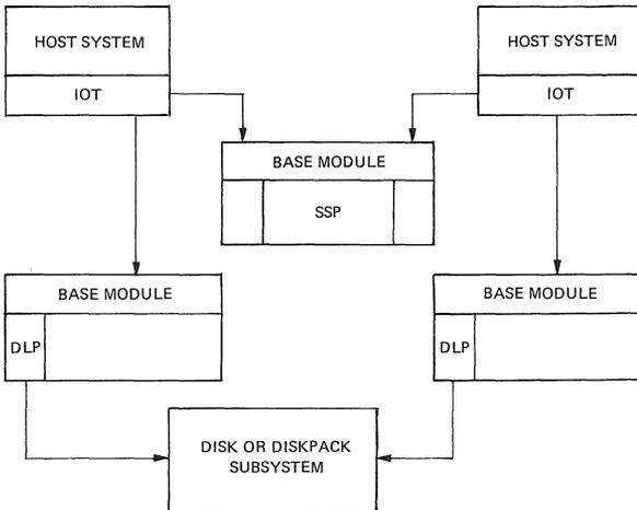
Figure 5-1. Typical Shared System Block Diagram
