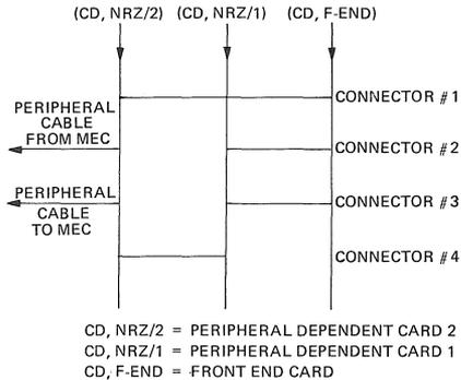
Figure 4-60. NRZ Tape DLP Frontplane Connectors
