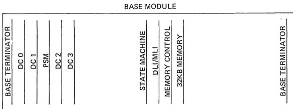
Figure 5-5. SSP Installed In An IOBC Base Module
