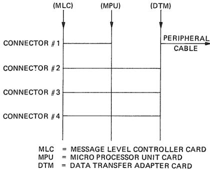
Figure 4-50. Uniline DLP Frontplane Connectors
