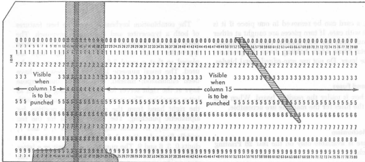
Figure 6. Card Visibility at the Punching Station
