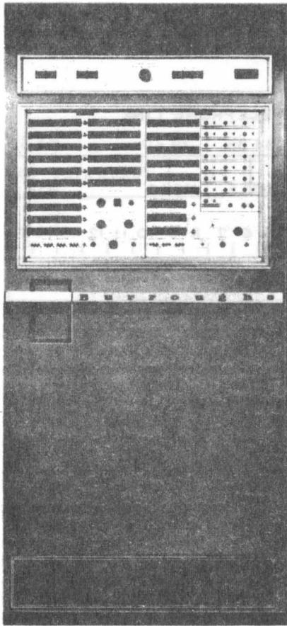
Figure 4-15. Controller-Comparator-Message Processor C-7122/GYK-10 (Message Processor Module On Right Side of Cabinet)
