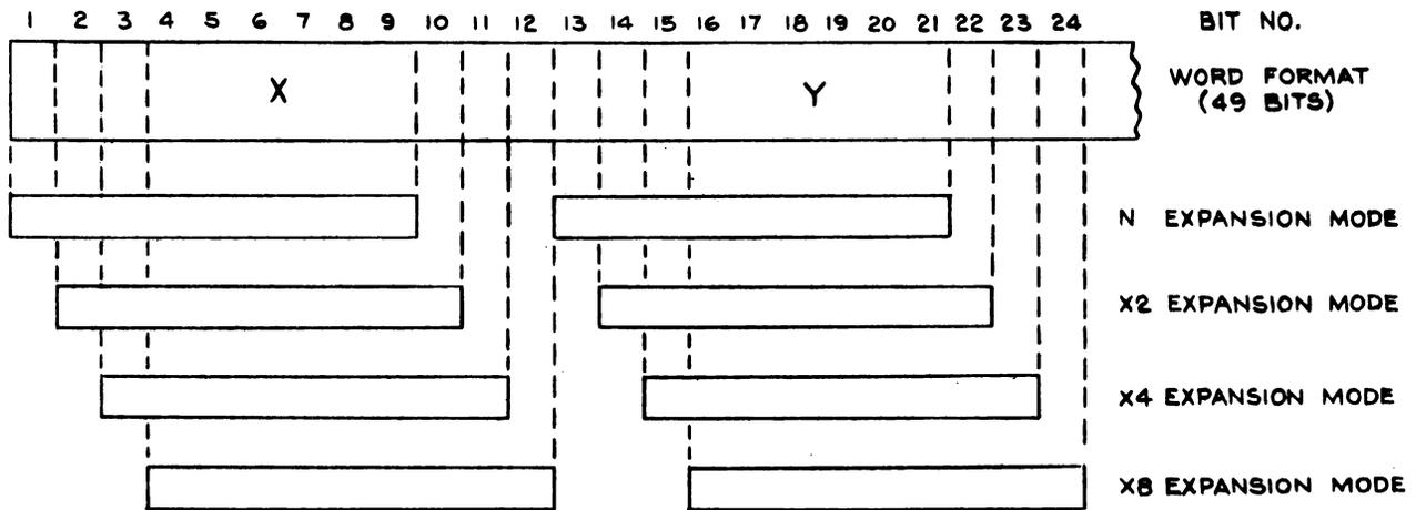
Figure 4-26. Gross-Position Bits of Input Message Used During X and Y Expansion Modes
