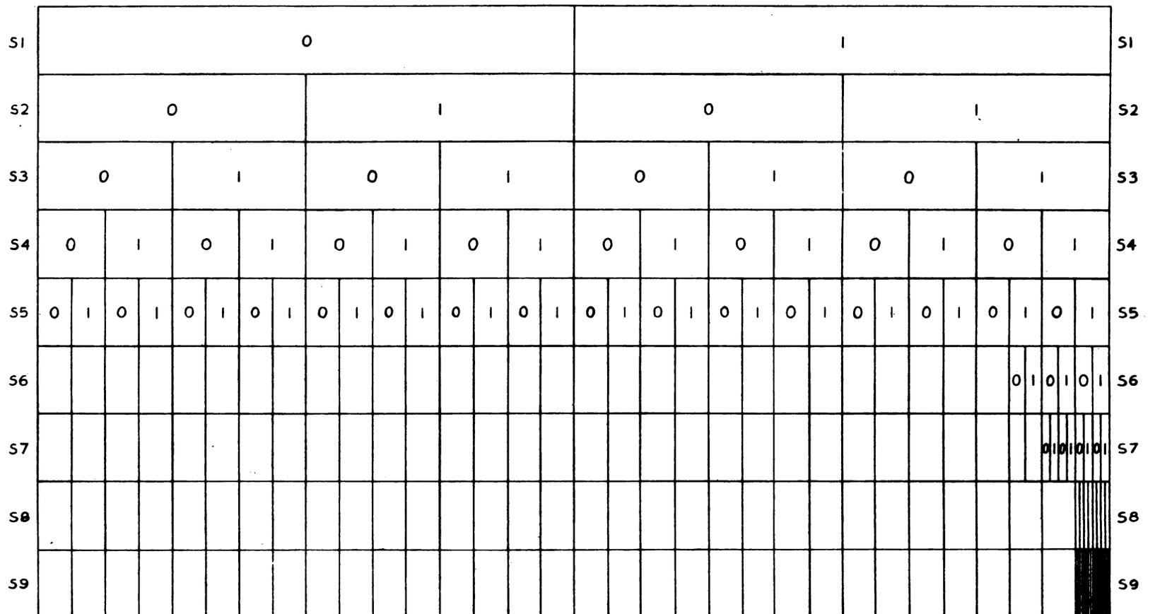
Figure 4-27. Gross-Position Division of Situation Display Screen
