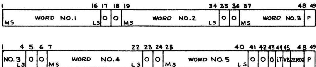
FORMAT OF MESSAGE IN OUTPUT STORAGE AREA OF THE MESSAGE PROCESSOR MODULE
