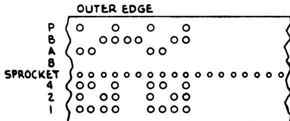
Figure 4-9. "Flexowriter" Paper-Tape Format
