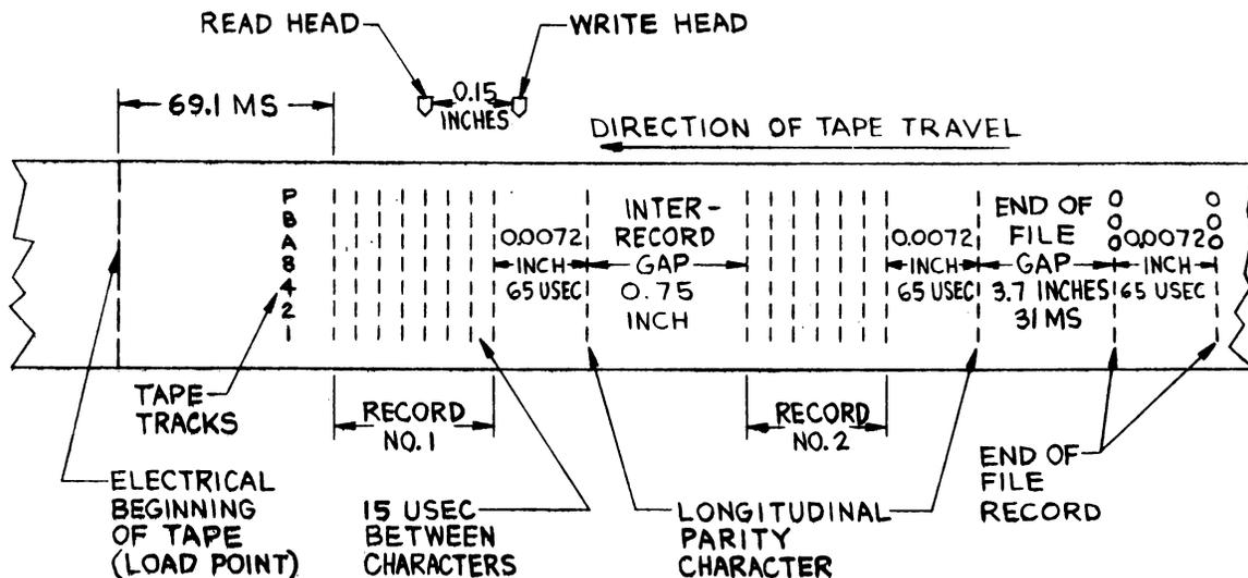
Figure 4-13. Magnetic Tape Format
