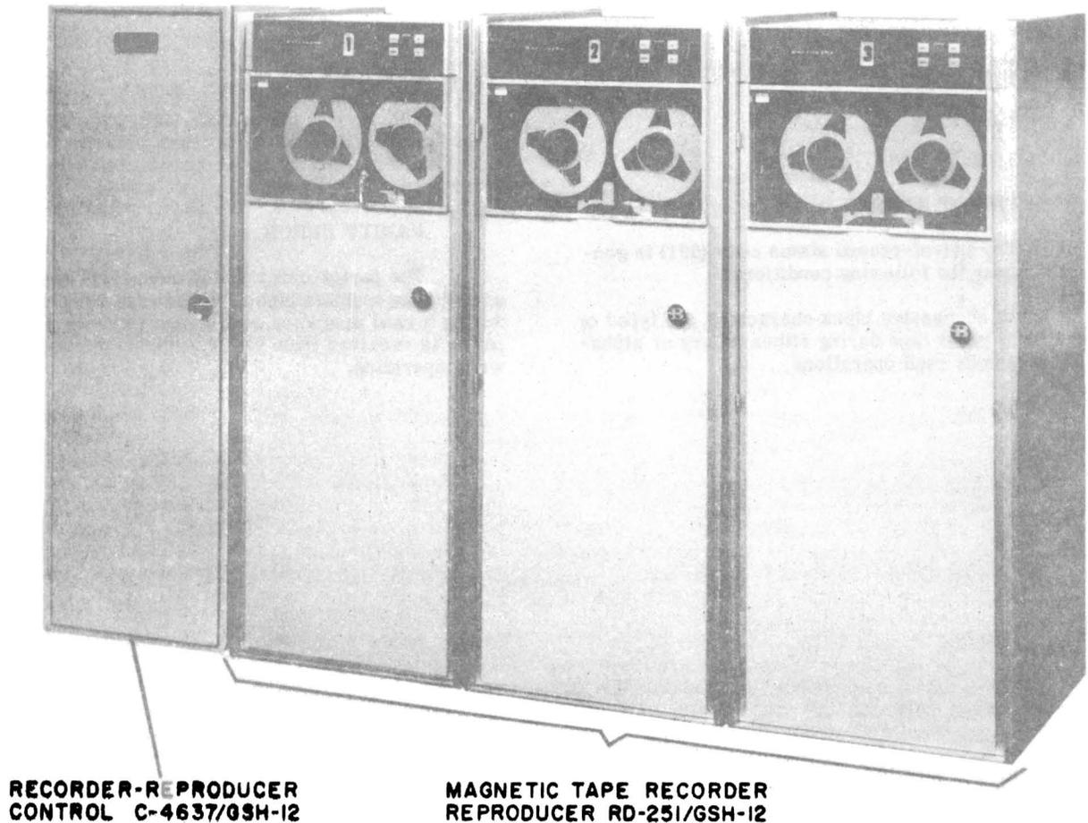
Figure 4-12. Magnetic Tape Recorder-Reproducer Set AN/GSH-22
