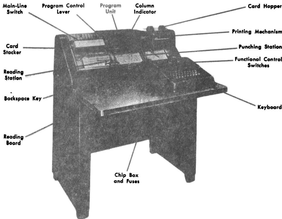
Figure 4. IBM 26 Operating Features
