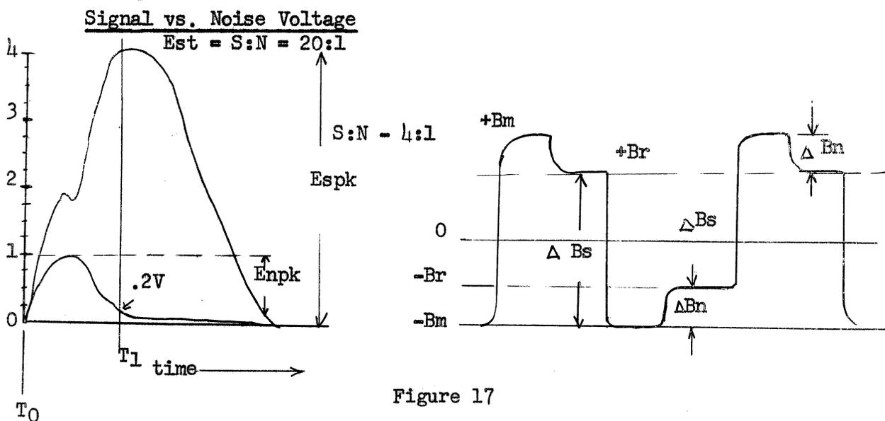
The  $Est$  signal to noise ratio may be obtained by reading the output (Tl) time from (T0) time zero. This sense time arrangement is usually incorporated in memory plane configurations rather than the conventional data processing and storage register circuitry. Chart 4 and Figure 13 may be studied as an indication of the Noise Signal Growth convictions. The
