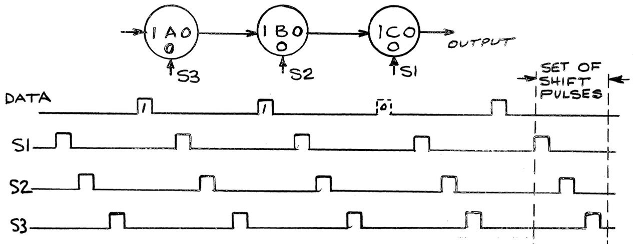
Figure 20 - Three Core Per Two Bit System and Timing
