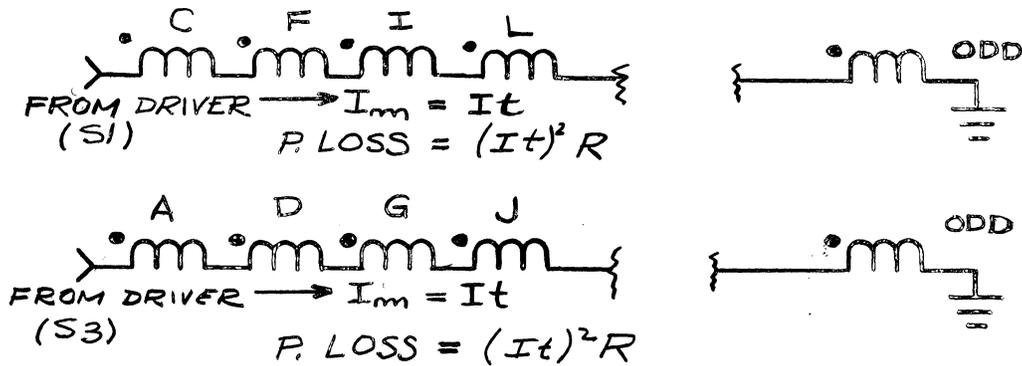
Figure 19 - Drive Winding Arrangement (series) for Figure 18
