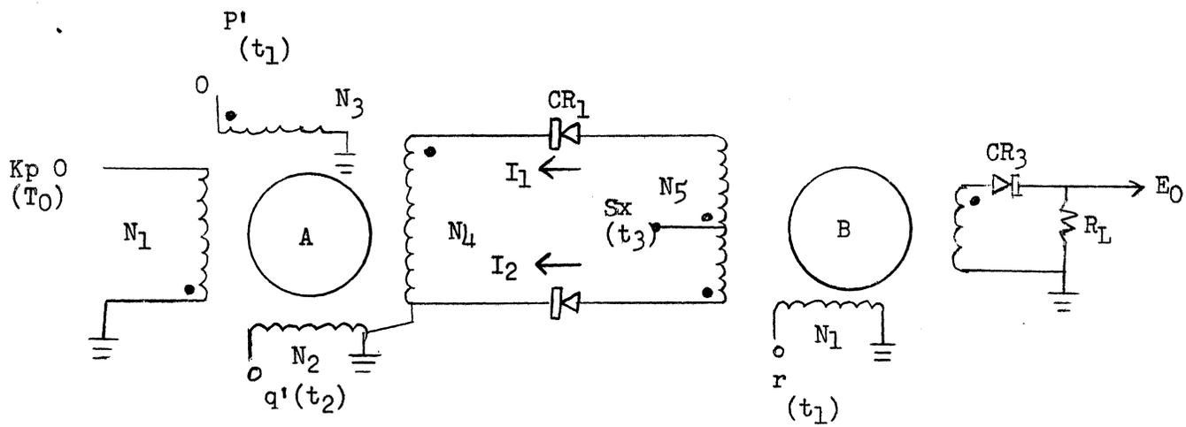
(a) Schematic of Double Diode Transfer Loop
