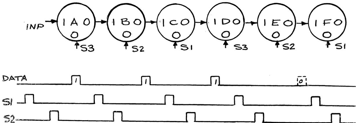
Figure 18 - Two Core Per Bit Shift Register and Timing
