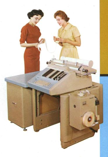
In some cases it is more feasible to punch tape as part of the alphanumeric accounting operation. Be sure to ask your Burroughs representative about the Burroughs F 1000 PA with A 520 Tape Perforator. This machine brings the same programming flexibility, automaticity, and accuracy to tape punching as the equipment discussed in this folder brings to the production of punched cards.
