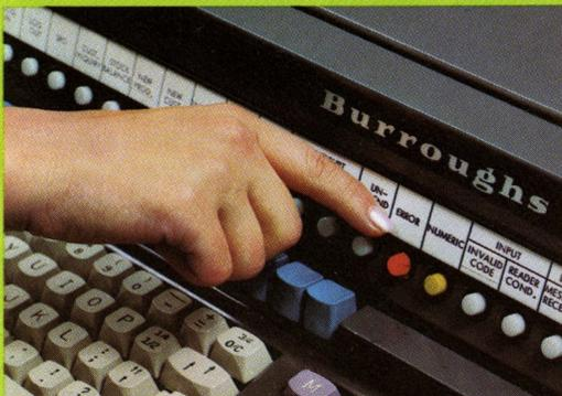
next, and indicate the status of data communications and the input/output peripherals. The error light and a bell activate when an input error is made, e.g., exceed capacity.
