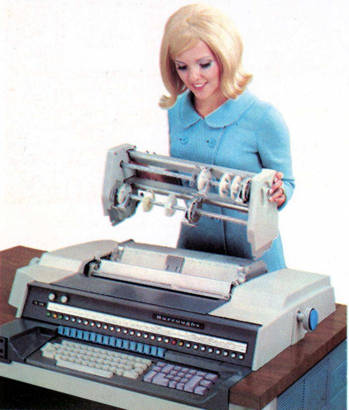
The TC 500 complements its high-speed printing capability with highly automated and flexible forms handling. Forms are spaced 6 lines per inch at speeds up to 20 lines per second. No external tapes or other mechanical control devices are needed. Spacing is completely controlled by internal programming.
