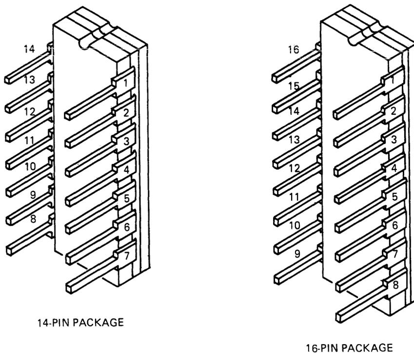
Fig. III-1 14 AND 16 PIN CHIPS
