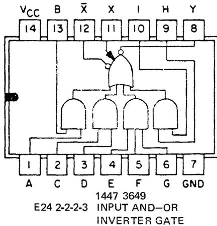
A high level is required at all inputs of a AND gate to produce a low level output from this circuit. A low level at any of the AND gate inputs produce a low level output from this circuit.
