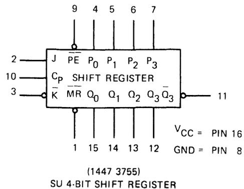
Fig. III-7 SU 4-BIT SHIFT REGISTER
