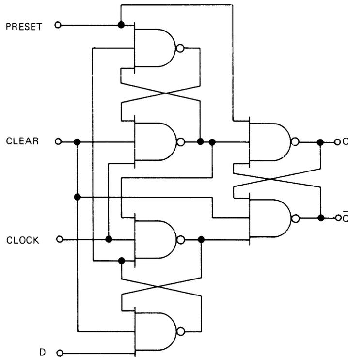
Fig. III-10 DF FUNCTIONAL LOGIC
