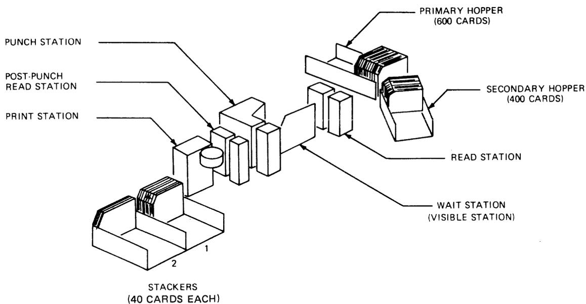
Fig. I-3 A9419-2 MECHANICAL LAYOUT
