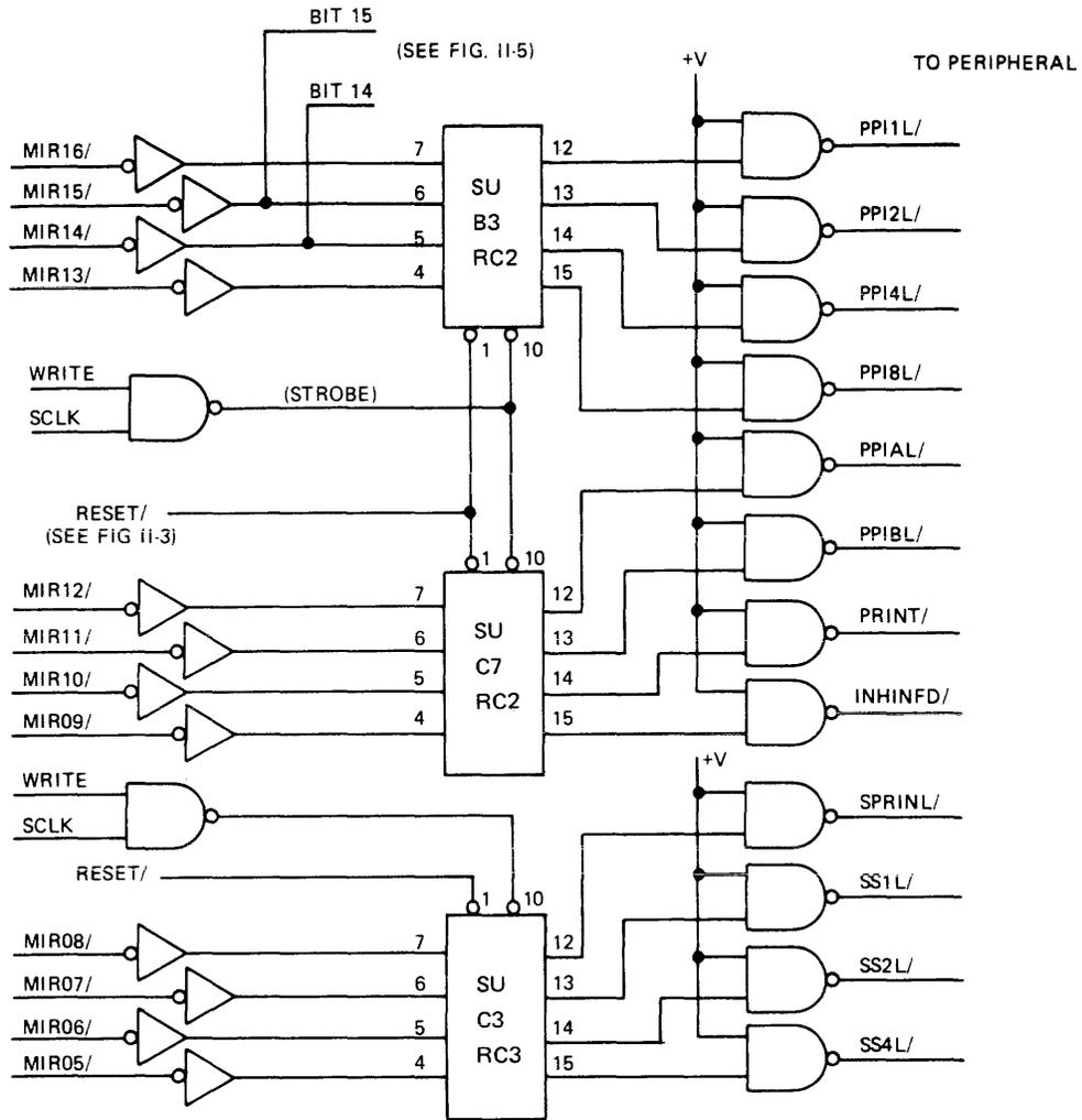
Fig. II-2 MOTION BITS/DATA BUFFER
