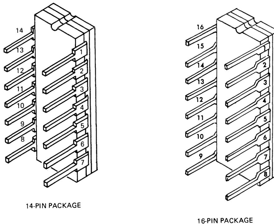
Fig. III-1 14 AND 16 PIN CHIPS
