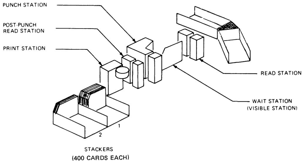
Fig. I-5 A9418-2 MECHANICAL LAYOUT
