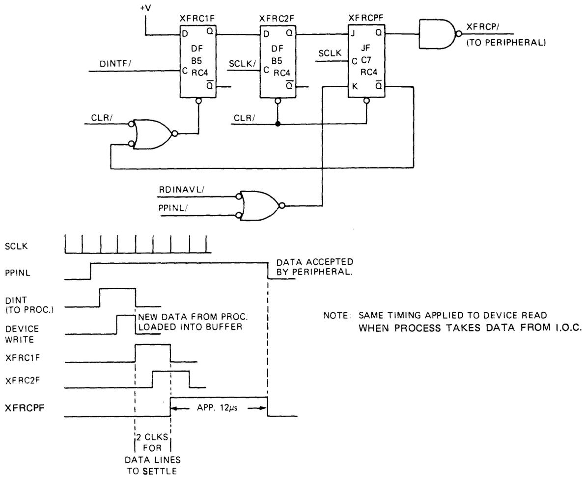
Fig. II-8 XFRCP CONTROL AND TIMING
