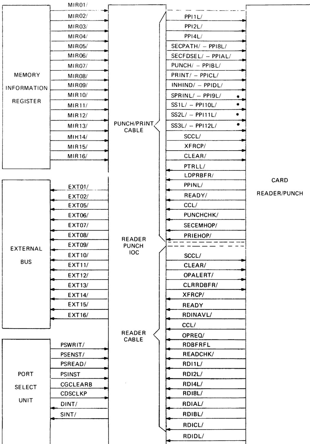
\* - SIGNALS PPI9L/ THROUGH PPI12L/ APPLY TO 80-COLUMN CARD PUNCH
