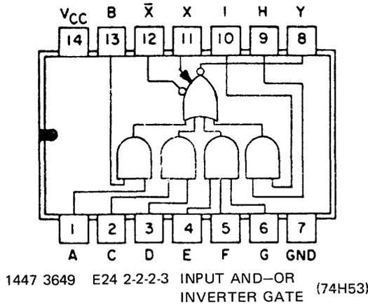
A high level is required at all inputs of a AND gate to produce a low level output from this circuit. A low level at any one input of each of the AND gates produces a high level output.
