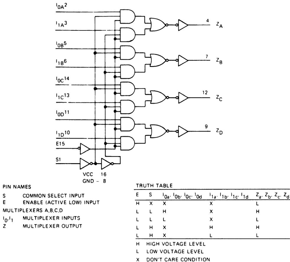
Fig. III-6 S2 QUAD 2-INPUT MULTIPLEXOR, FUNCTIONAL LOGIC AND TRUTH TABLE
