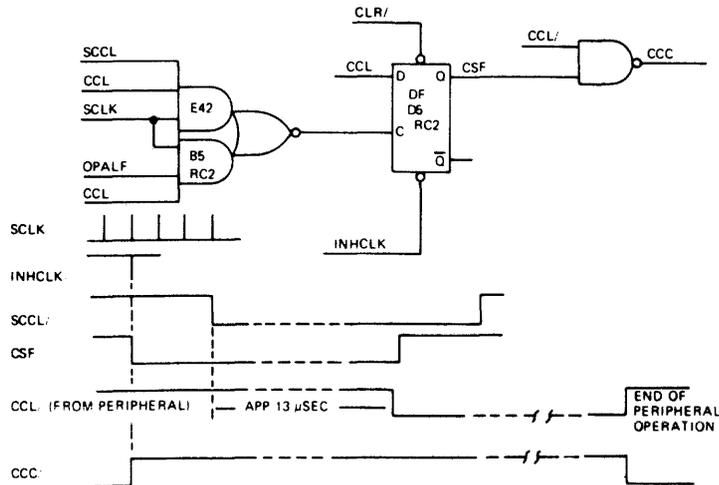
Fig. II-4 CSF, CCC/ AND TIMING
