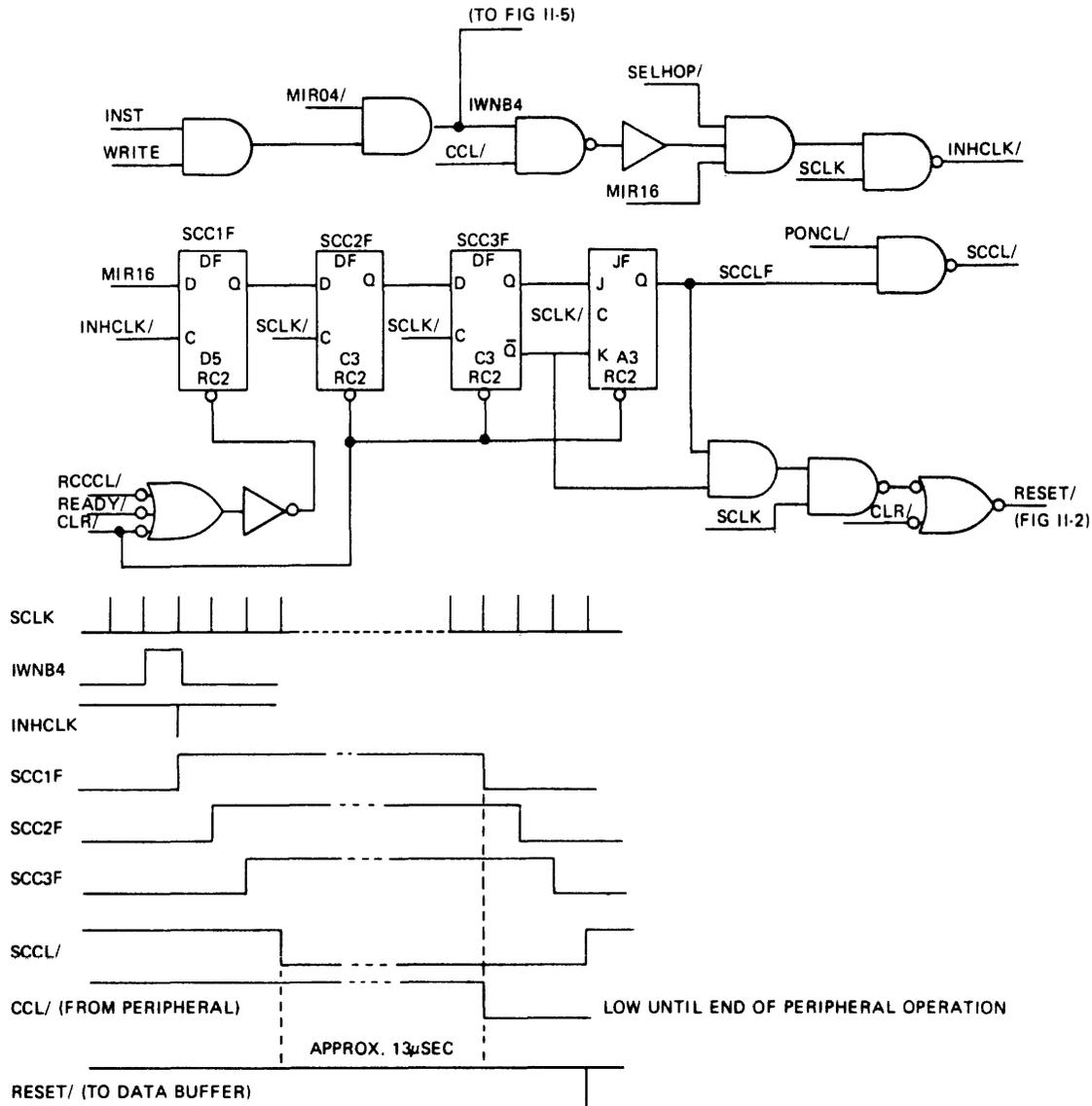
Fig. II-3 INHCLK, SCCL GENERATION AND TIMING
