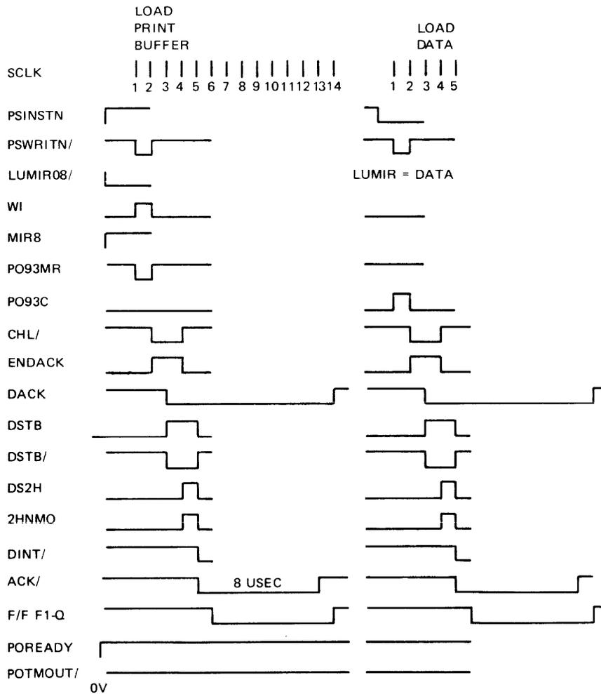
TIMING CHART II-1 LOAD PRINT BUFFER TIMING
