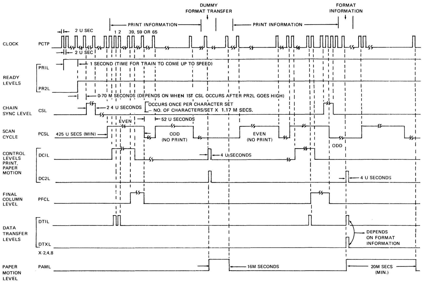
Fig. II-10 TIMING DIAGRAM FOR 400 LPM PRINTER
