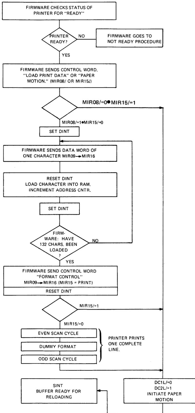
Fig. II-3 BUFFER LOAD AND PRINT OPERATION
