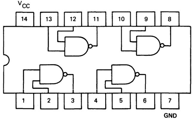
Fig. III-1 TWO-INPUT POSITIVE NAND BUFFER (1447 9596) AND TWO-INPUT POSITIVE NAND GATE (1447 0240)
