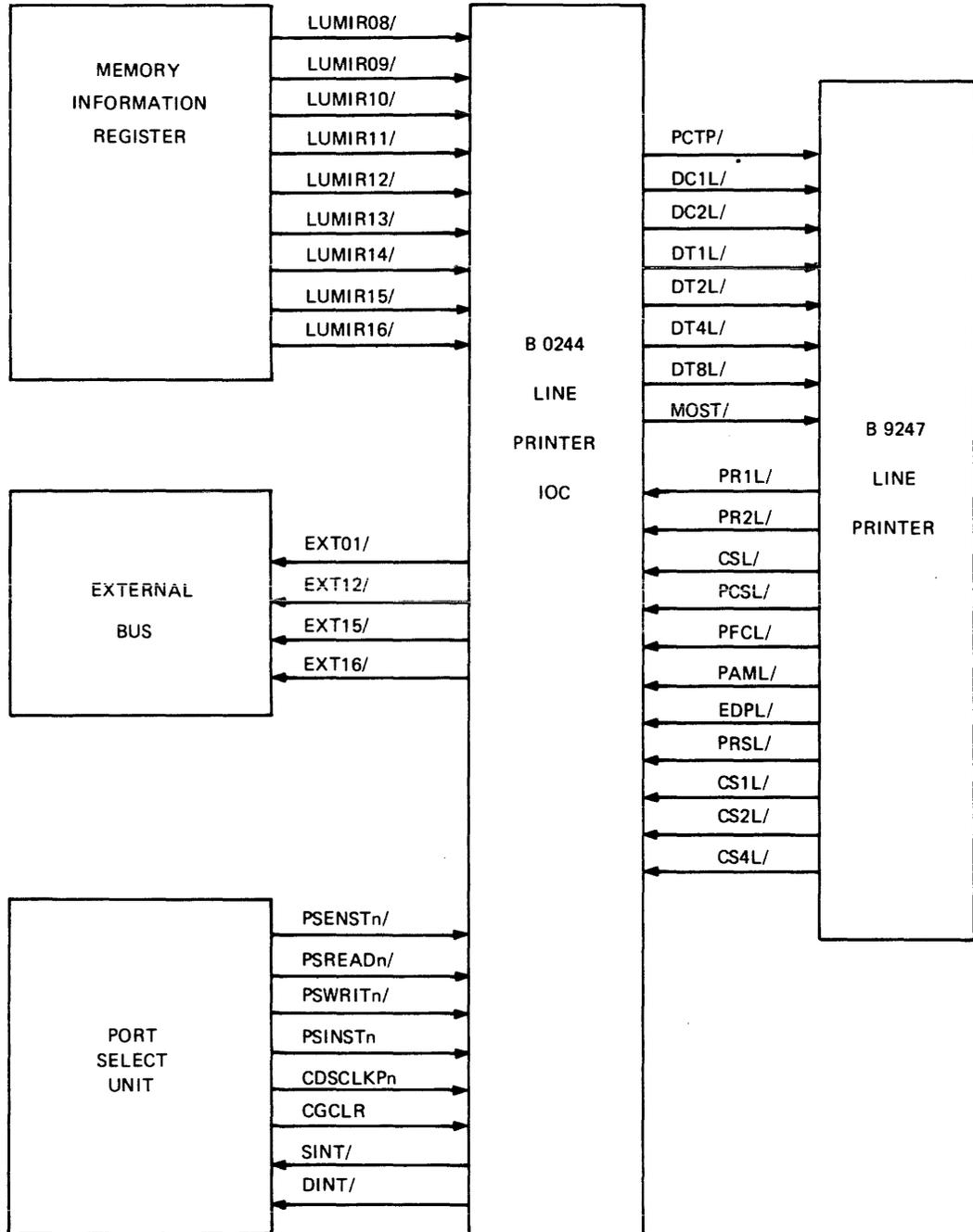
Fig. I-1 INTERFACE BLOCK DIAGRAM
