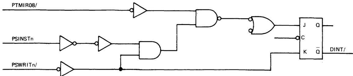
Fig. II-6 DINT FROM LOAD BUFFER CONTROL WORD
