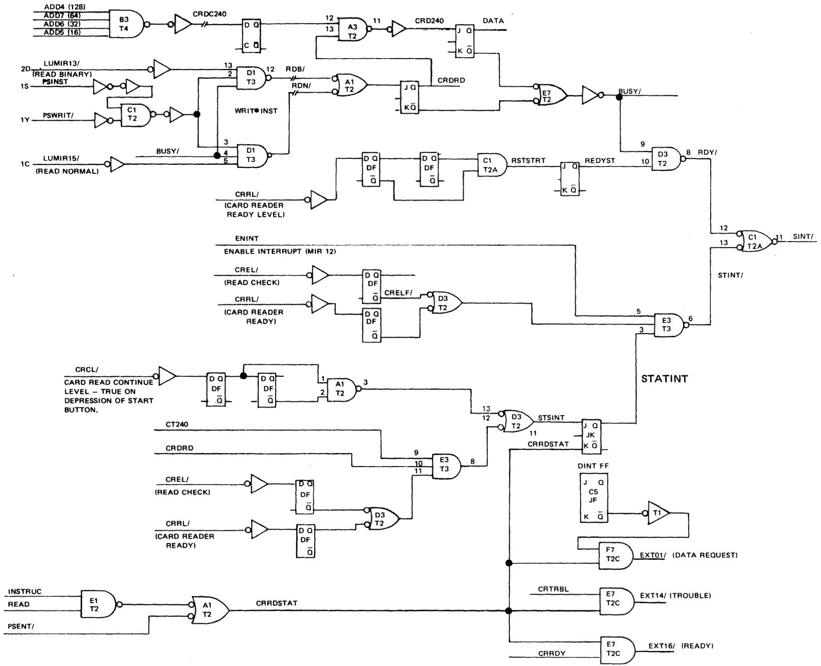
Fig. II-5 STATUS INTERRUPT, LOGIC DIAGRAM
