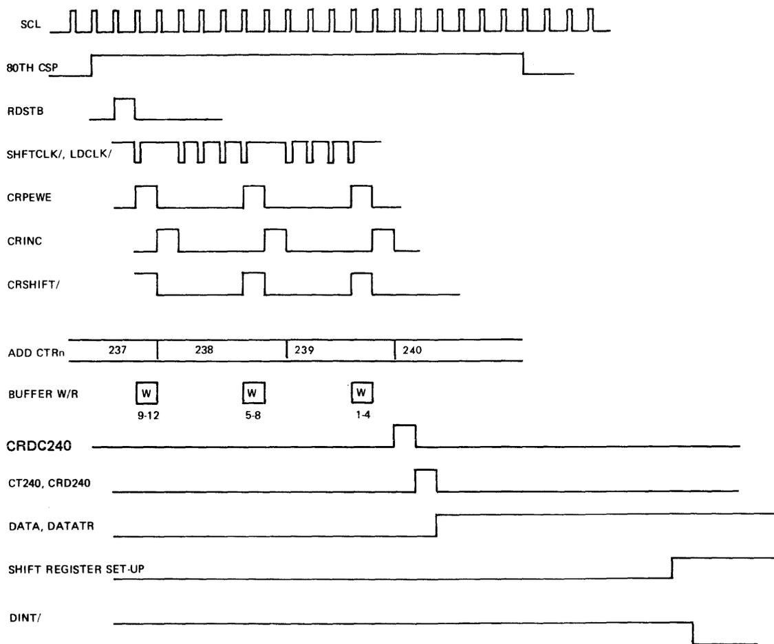
Fig. II-3 BUFFER LOAD TIMING FOR LAST COLUMN
