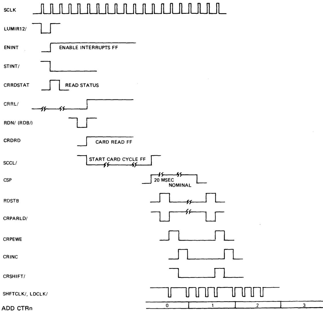
Fig. II-2 BUFFER LOAD TIMING, FIRST COLUMN
