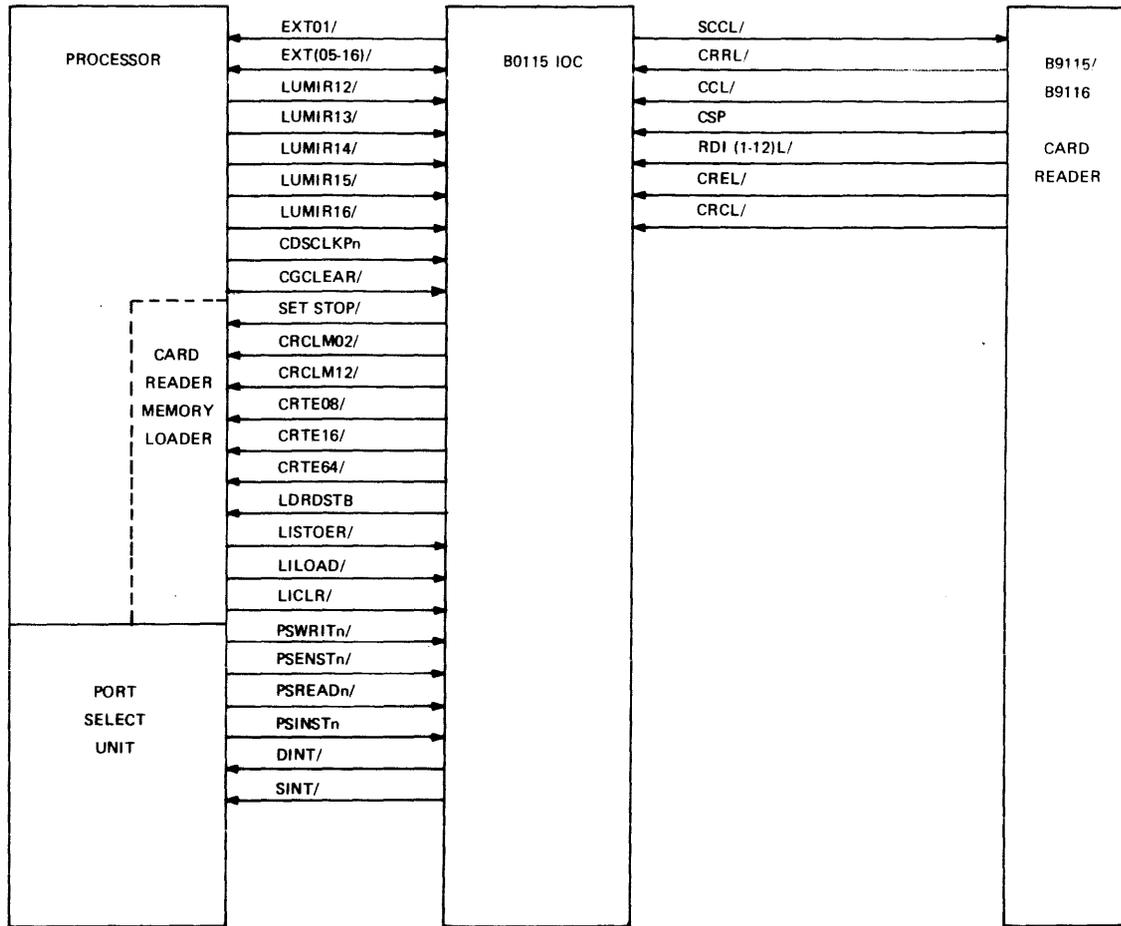
Fig. I-2 B0115 CARD READER IOC SIGNAL INTERFACE, BLOCK DIAGRAM
