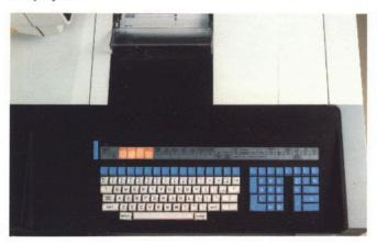
The *inbuilt printer* produces forms which are 8.5 inches (22.6 cm) wide—easy to work with and precisely the convenient size for most filing systems. Its 90 characters-per-second matrix printer is bi-directional for fast throughput.
