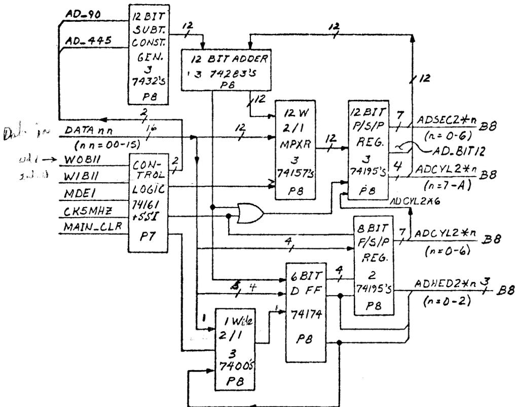
Figure 1-7. Address Decoder
