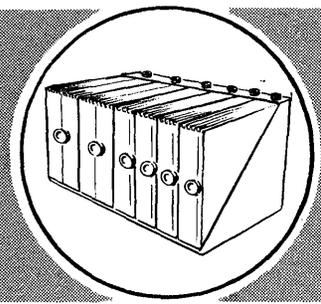
boards. At final assembly, the printed circuit board is inserted into a grooved trough on the inside edge of the holder; the other end of the board is then fitted over the connector pins that protrude slightly above the p. c. board. The pin-to-board connection is then rigidly fixed by dip-soldering the assembly, thus ruggedizing the circuit network module. Heat is removed directly from the flat-pak source via an interface between the flat-pak and the aluminum carrier.
