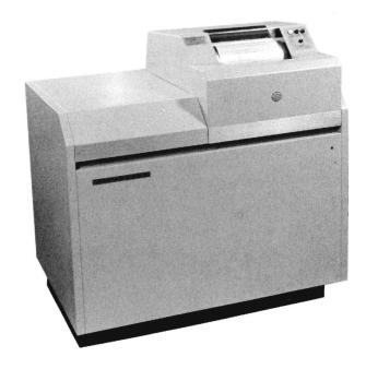
paper. Under continuous operation, a line of printing is visible two seconds after recording.
