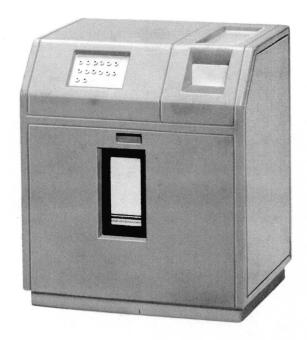
Invalid characters are sensed and replaced by six zero bits and an error indication is supplied to the computer. Binary codes are read column by column, six bits at a time. Since there are 12 bits in a binary column, each card column occupies the equivalent of two six-bit characters.
