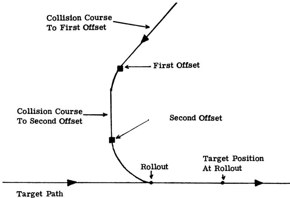
Figure 10-8. Double-Offset Stern Attack
