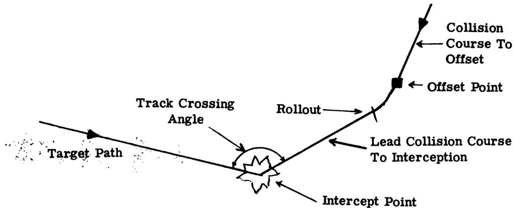
Figure 10-13. Front and Beam Final Turn Attacks
