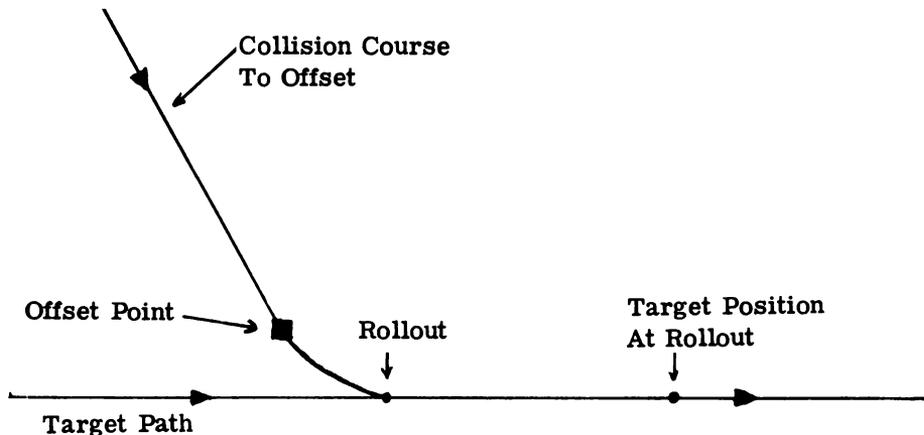
Figure 10-7. Single-Offset Stern Attack
