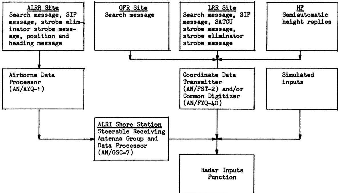
Figure 4-1. Data Types and Sources for Radar Inputs Function
