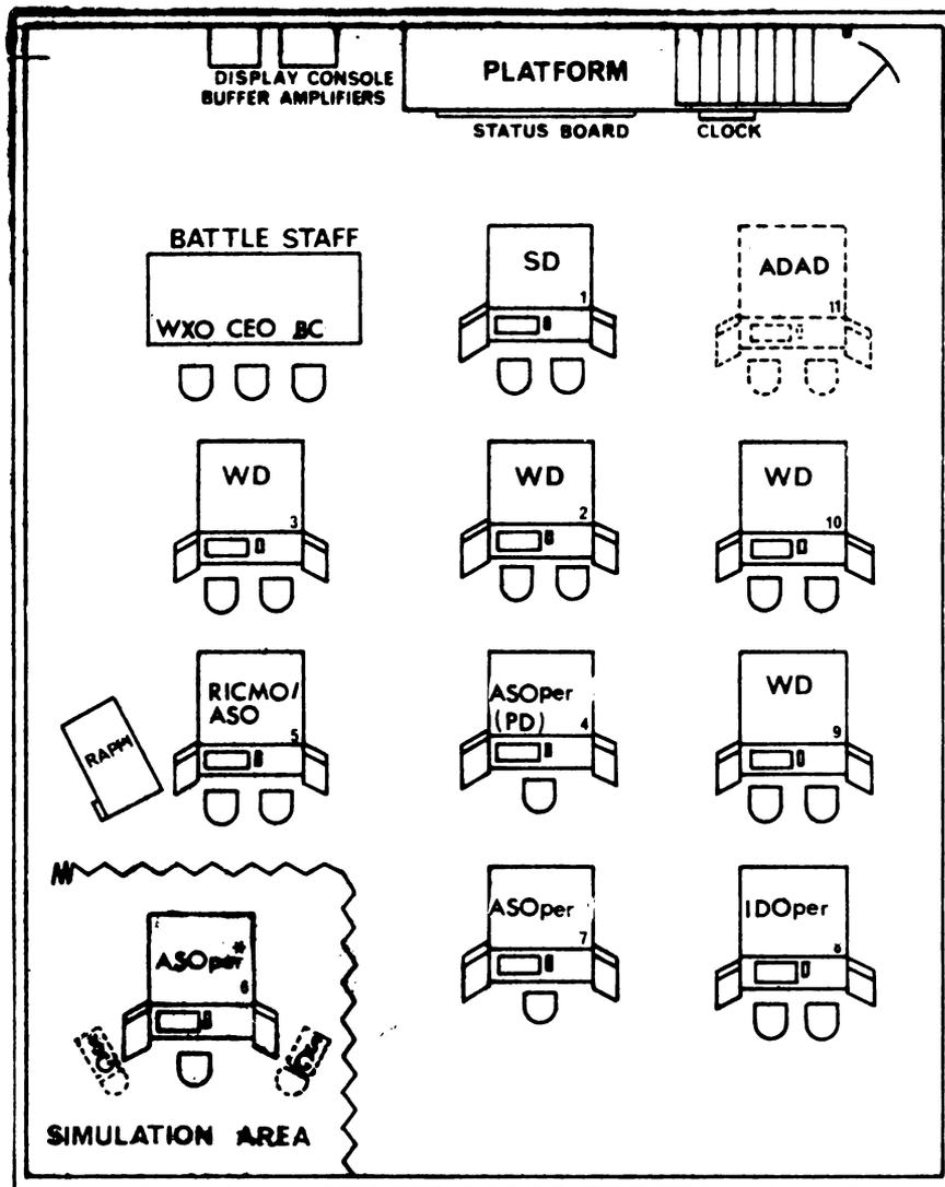
\*During simulation exercises, console 6 is manned by a Simulation Supervisor (SIM SUP), and two Interceptor Pilot Simulators (IPSS) who operate the simulator group (SG) manual input keyboards.
