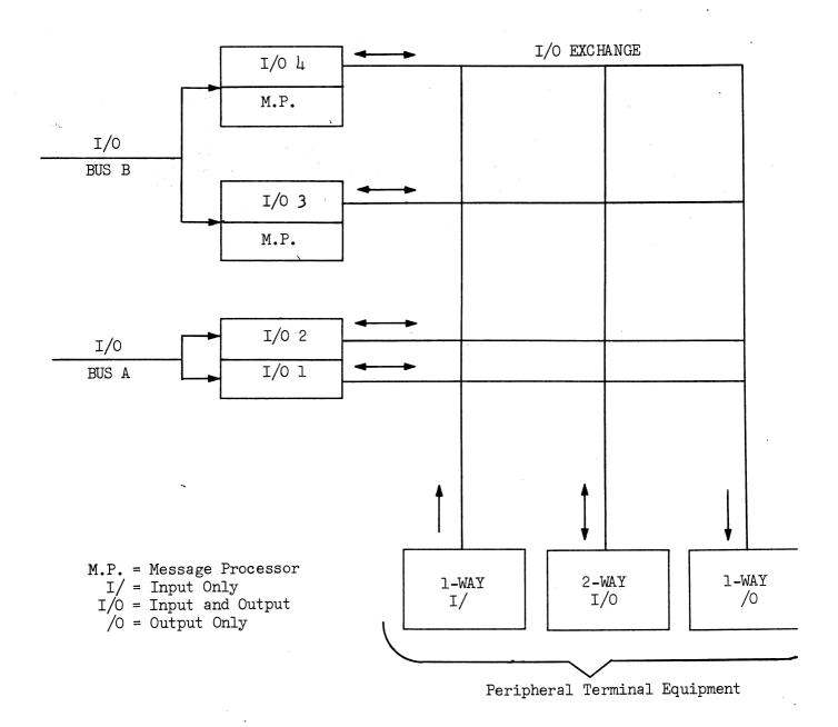
Figure 2, INPUT/OUTPUT EXCHANGE
