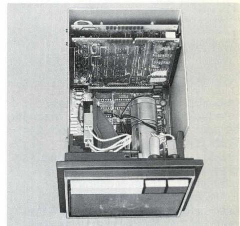
The drive accepts write data and drive commands and provides read data and status information to the host. The in-built microprocessor interprets commands and moves the tape as required while controlling tape speed and tension. Status information generated from sensors within the drive is also handled by the microprocessor.
