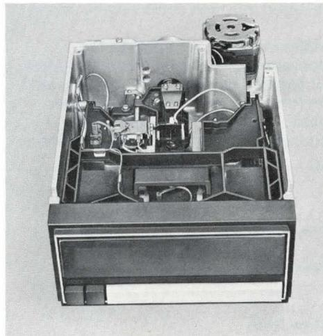
With 1.25 megabytes of fast random access storage, the 9489 is well suited for computer based, transaction-oriented small business systems and intelligent terminals. In the dual drive Master/Slave configuration, the Master connects via an I/O cable to the host and contains additional electronics common to both units. The Master and Slave units are interconnected and allow for seek/overlap operations and a combined storage capacity of 2.5 megabytes.
