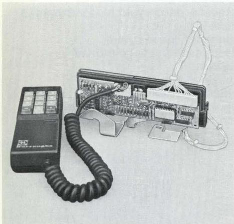
In-built LSI circuitry enables easy interfacing to host equipment. Magnetic stripe data read from either Track 2 or Track 3 is processed internally, including extensive data checking, and presented to the host as buffered parallel-bit, TTL-level characters. Self-synchronous circuitry accommodates card speeds over the range of 8 to 100 inches per second.
