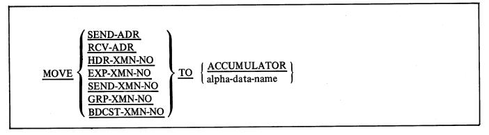
Option 6 is used to retrieve the various address and transmission numbers from the adjunct exchange memory.
