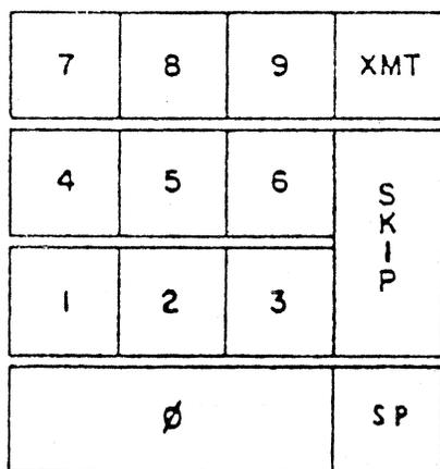
**Figure 4-3. 10-Key Auxiliary Keyboard**
