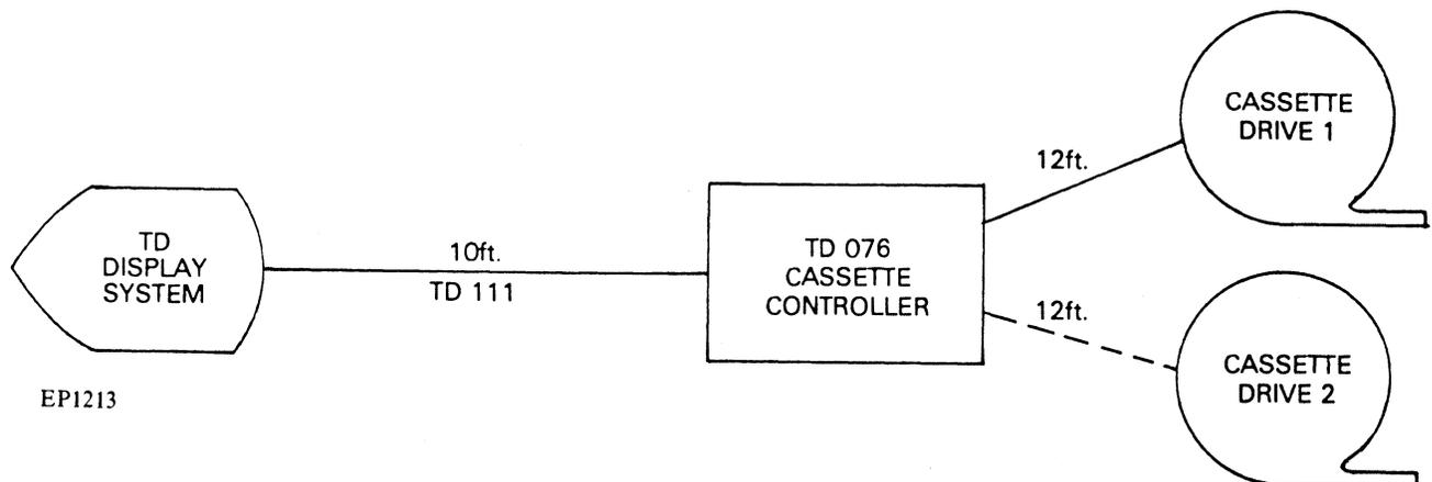
Figure 7-1. Single TD/Cassette Controller Configuration
