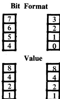
As indicated in table A-1, setting bits 1, 2, 3, 5, 6 to the ONE state results in the hexadecimal value of 6E.
