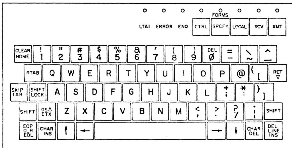
Figure 4-1. U.S. Typewriter Keyboard, ASCII
