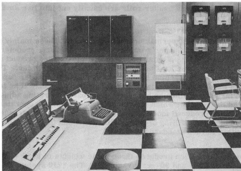
IBM 1710 PROCESS CONTROL SYSTEM which supervises papermaking at Cellulose du Pin's Factice plant, is centered around an IBM 1620 COMPUTER (console at left). Unit at right of window is a French-made analog signal indicator which continuously feeds the computer production line data.
