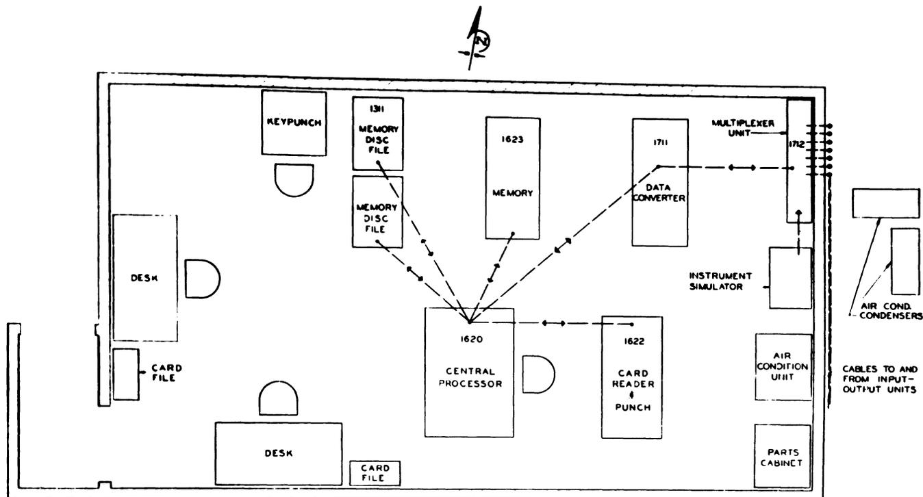
Fig. 3 - CONTROL SYSTEM COMPUTER ROOM, located close to the electric furnaces, is air conditioned and pressure-tight. An emergency air conditioning system is available on a standby basis.
