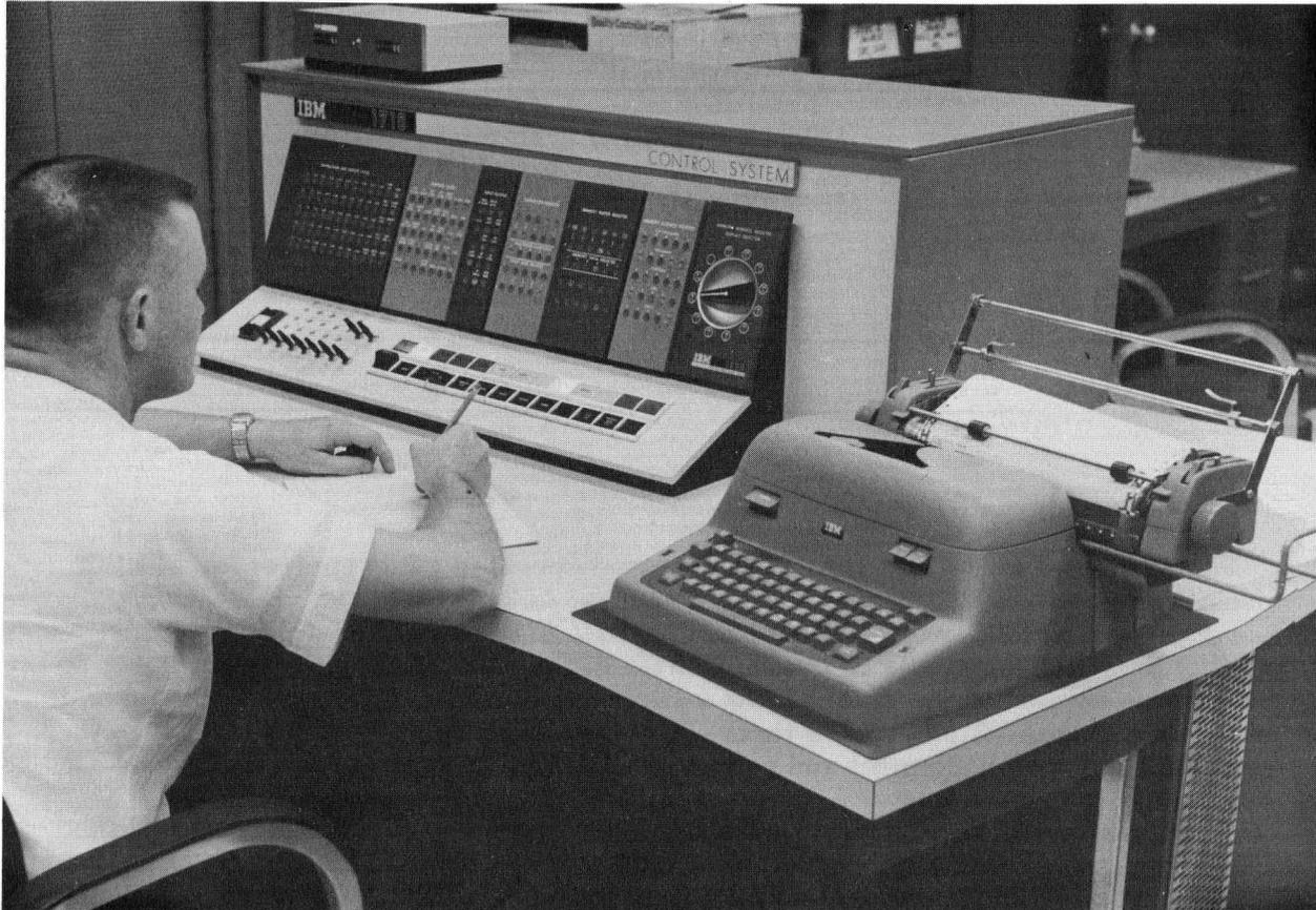
Fig. 1 - IBM 1710 CONTROL SYSTEM at Lukens Steel (IBM 1620 processor shown here) implements the first known on-line computer tie-in with large electric steel melting furnaces.
