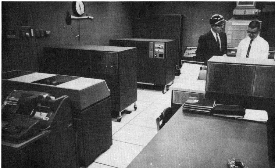
Fig. 2 - IBM 1710 SYSTEM CONFIGURATION is centered around an IBM 1620 processor (far right). Two IBM 1311 magnetic disc files (behind keypunch) expand mass memory. Linkage to instrument sensors and input units and conversion of analog signals are provided by IBM 1712 multiplexer (in corner against back wall) and IBM 1711 data converter (in front of 1712).
