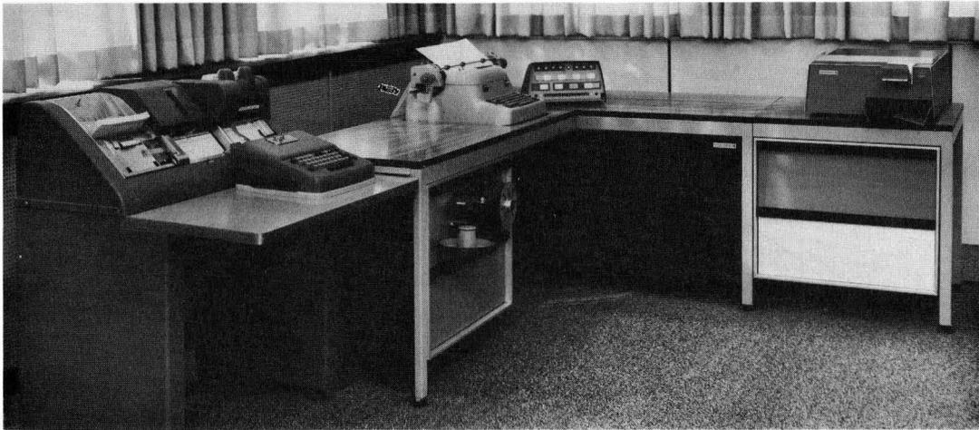
Fig. 1. - MONROBOT XI in its vendor quality rating configuration uses punched card input prepared on IBM 026 keypunch (shown at left). Monro-Card Processor is on top surface right.
