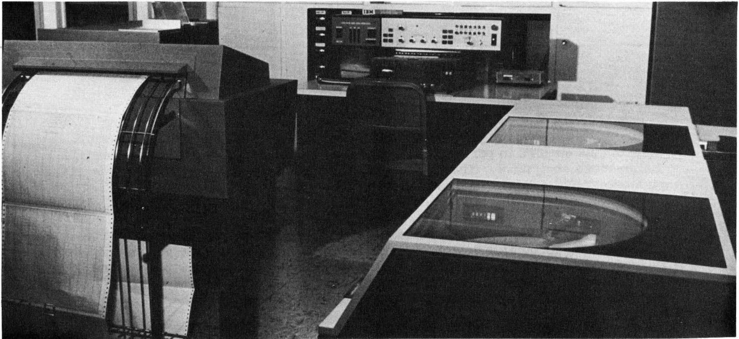
Fig. 1. IBM 1440 DATA PROCESSING SYSTEM used by Sigman includes IBM 1443 card read-punch (upper left), IBM 1443 printer (lower left) and two IBM 1311 disc drives (lower right).
