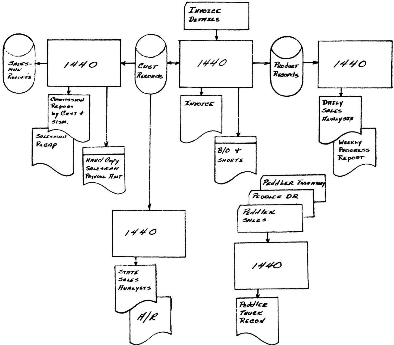
Fig. 3. SIGMAN BILLING SYSTEM fulfills invoicing requirements and provides input to salesmen's commissions payroll.
