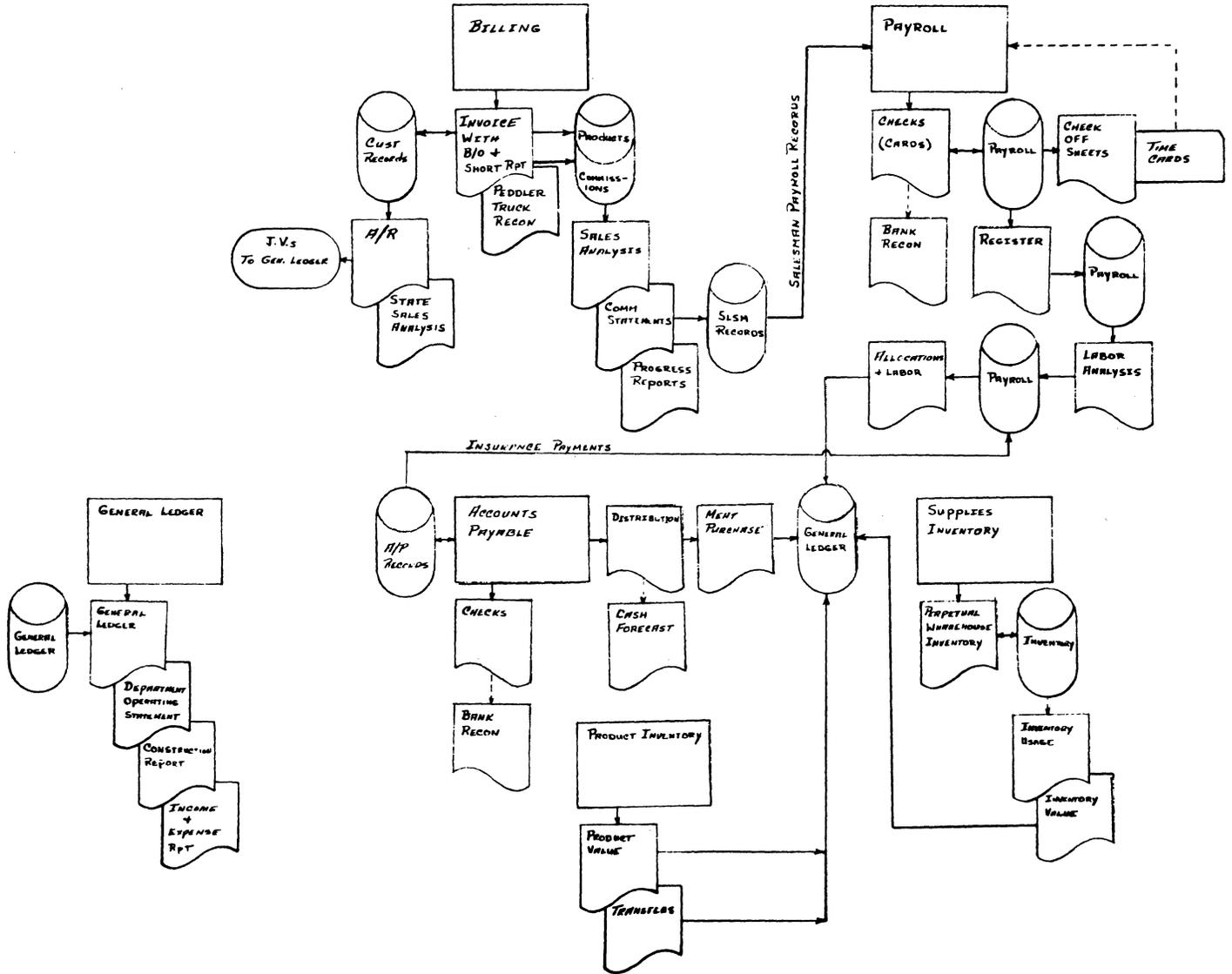
Fig. 2. SIGMAN TOTAL SYSTEM FLOW CHART shows integration of all company functions into a single, unified system.
