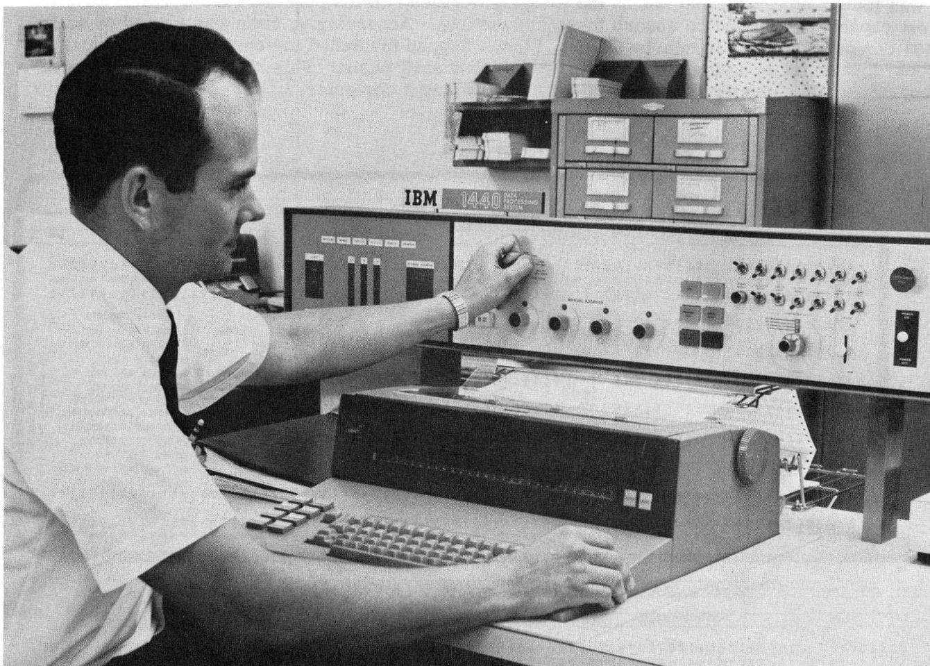
**Fig. 1. IBM 1440 DATA PROCESSING SYSTEM** covers for Tappan such important areas as production and inventory control and sales analysis.
