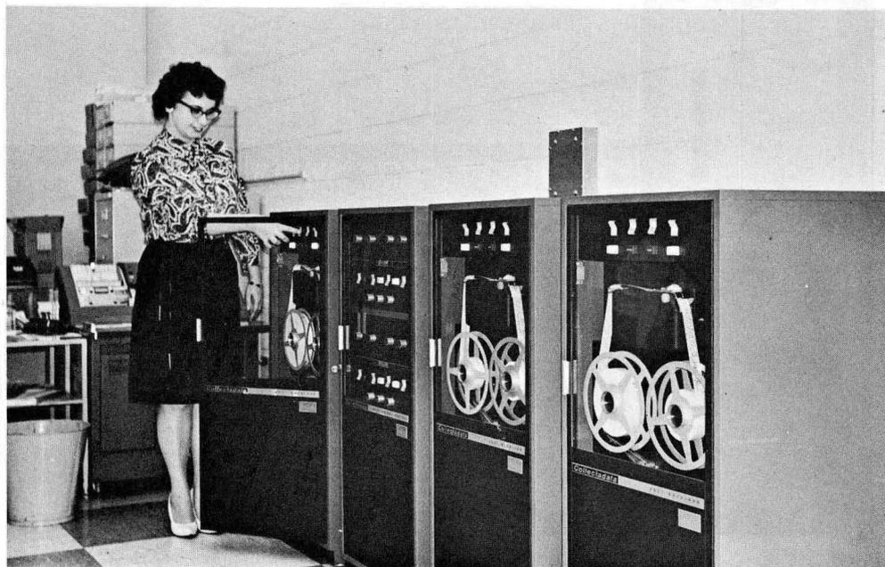
OPERATOR PREPARES TO LOAD A REEL OF PAPER TAPE IN THE RECEIVER CONSOLE. ADJOINING UNIT IS THE CENTRAL CONSOLE.
