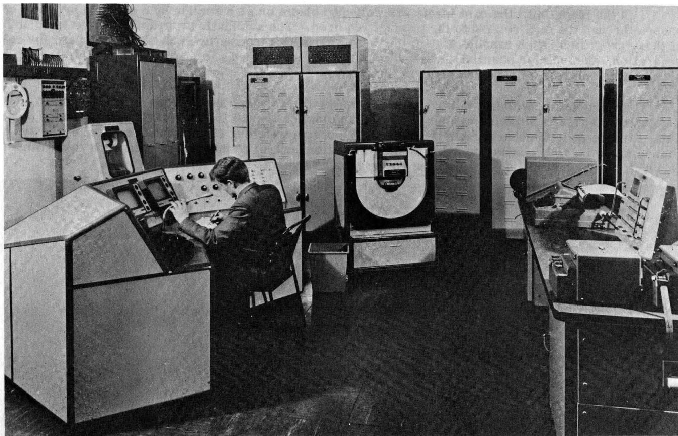
PRODUCTION CONTROL CENTER AT PARK GATE. THE OPERATOR CAN GIVE INSTRUCTIONS TO THE COMPUTER OR TALK TO MILL CREWS THROUGH MICROPHONE.
