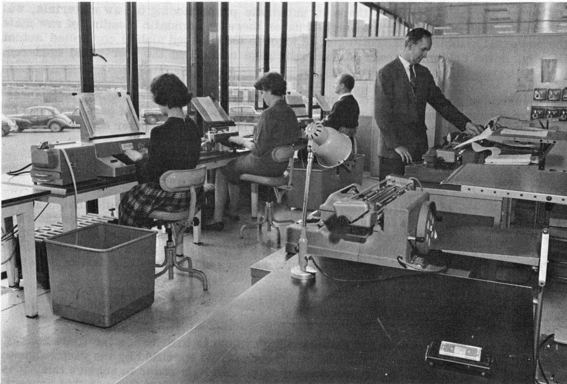
OPERATORS CHECKING INFORMATION INCLUDED ON PAPER TAPES WHICH IS TO RELAYED TO THE GE-412 COMPUTER.
