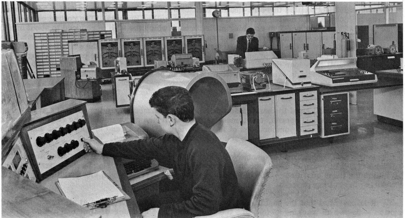
COMPUTER CENTER. OPERATOR IN FOREGROUND AT CONSOLE OF INGOT AND SLAB CONTROLLER CAN INTERROGATE ELLIOTT 803 COMPUTER TO OBTAIN AN UP-TO-DATE STATUS OF THE PLANT.
