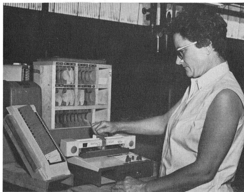
AN OPERATOR MAKES A RECORDING ON THE DATA COLLECTION DEVICE. PERSONNEL CARDS AND INDIRECT SET UP AND OVERTIME EXCESS CARDS ARE IN THE RACK TO THE LEFT. THE CARD AND STORAGE RACKS ARE IN THE BACKGROUND.
