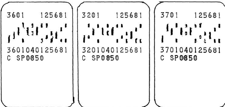
PRODUCTION MASTER PLASTIC CARDS CONTAIN THE ACCOUNT NUMBER AND PRODUCTION ORDER NUMBER ON THE FIRST LINE, ACCOUNT NUMBER, TRANSACTION CODE (040) AND PRODUCTION ORDER NUMBER ON THE SECOND LINE AND STOCK, PART, OR CATALOG CODE AND NUMBER ON THE THIRD LINE. THERE IS ONE CARD FOR EACH DEPARTMENT ON THE PRODUCTION ORDER.
