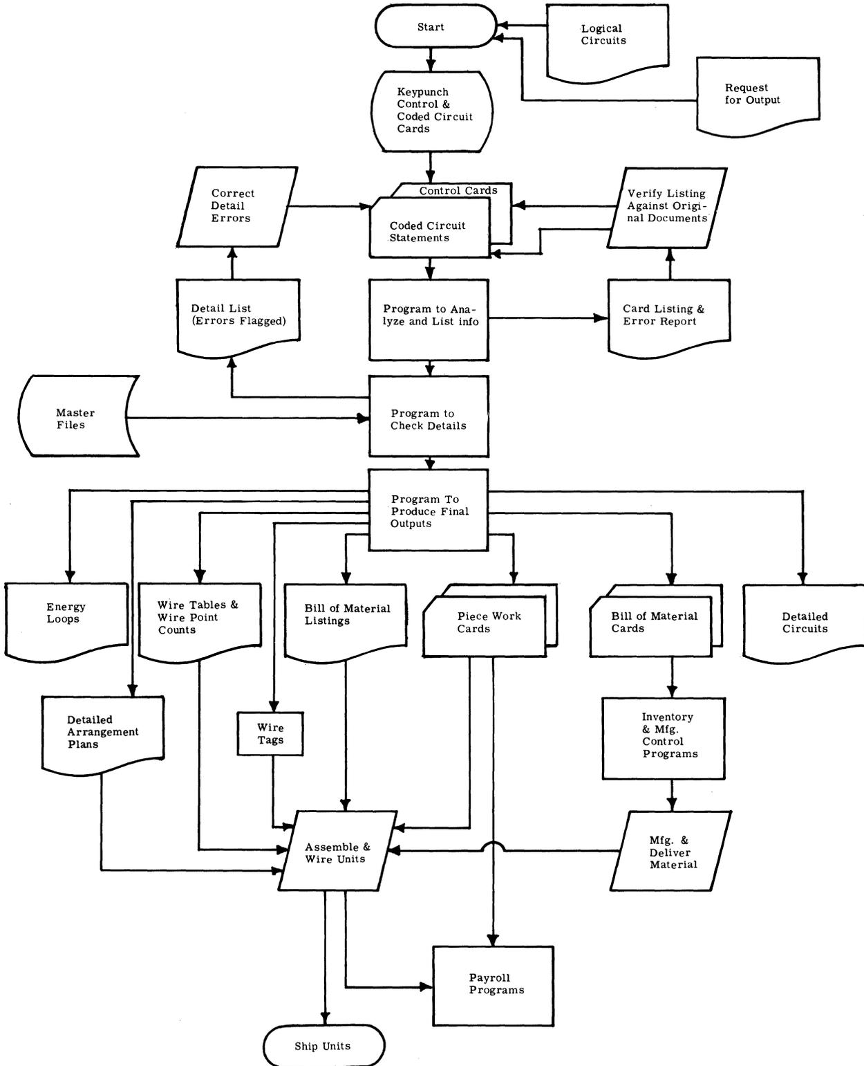
FROM TWO PRIMARY INPUT SOURCES, LOGICAL CIRCUITS AND REQUEST FOR OUTPUT, THE PROGRAMS ARE DESIGNED TO PRODUCE EIGHT MAIN OUTPUTS USED IN THE ASSEMBLY OF GENERAL RAILWAY'S SIGNAL'S PRODUCTS AND FOR SUBSEQUENT APPLICATIONS INCLUDING INVENTORY CONTROL AND PAYROLL.
