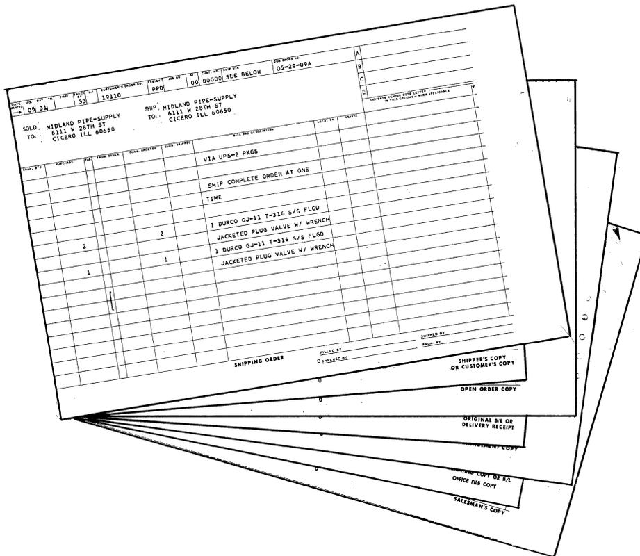
THE MULTIPART FORM--PICKING ORDER, BILL OF LADING, SHIPPING ORDER AND OFFICE CONTROL COPY, ETC.-- IS GENERATED BY THE FIRST PASS OF CARDS. SECTIONS STAY WITH THE GOODS TO THEIR DESTINATION: OTHER SECTIONS RETURN TO THE OFFICE WITH FIGURES FOR AMOUNTS ACTUALLY SHIPPED TO BE PUNCHED INTO CARDS FOR SECOND MACHINE PASS.
