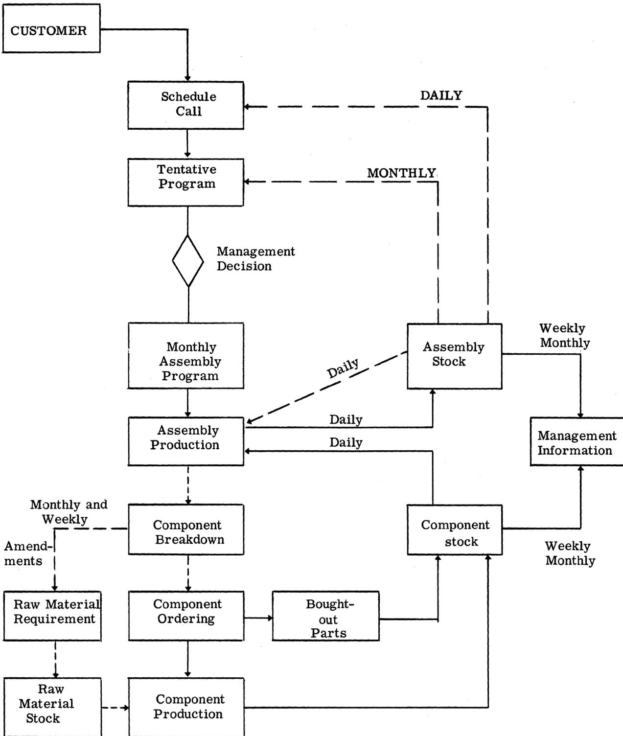
THIS DIAGRAM SHOWS THE INFORMATION FLOW OF THE PRODUCTION CONTROL SYSTEM WHICH, IN ADDITION TO PROVIDING PRODUCTION SCHEDULING INFORMATION FOR ASSEMBLY BUILD, COMPONENT PRODUCTION AND BOUGHT-OUT MATERIALS, PROVIDES SENIOR MANAGEMENT WITH CONTROL DATA ON STOCKS AND PRODUCTION ACHIEVEMENT. STOCK CONTROL TECHNIQUES ARE USED IN SUPPORT OF BOTH THE ASSEMBLY AND COMPONENT ORDERING SYSTEMS.
