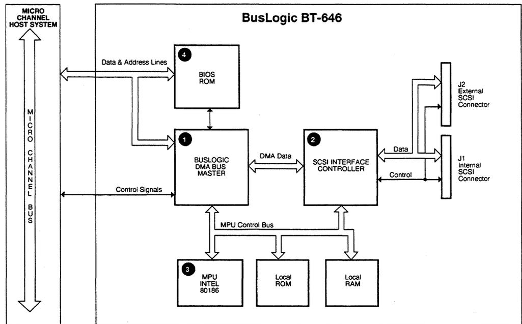
Figure 1-2. Host Adapter Architecture
