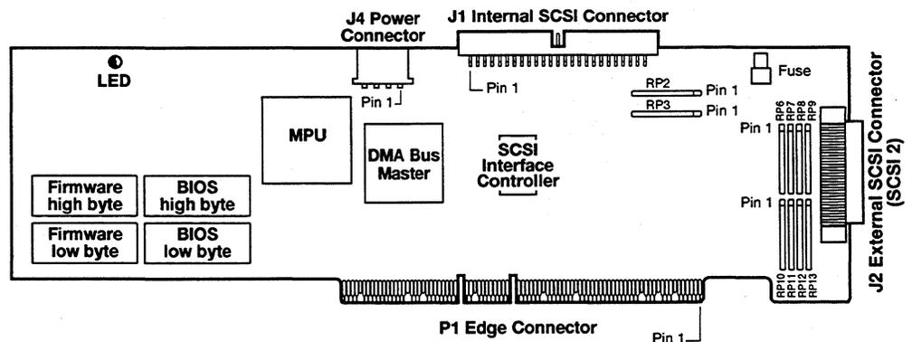
Figure 2-1. The BT-646 Host Adapter Board
