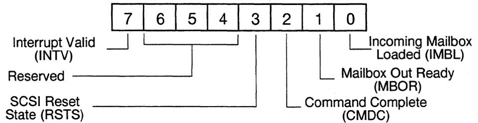
Figure 4-5. Interrupt Register (Read Only)
