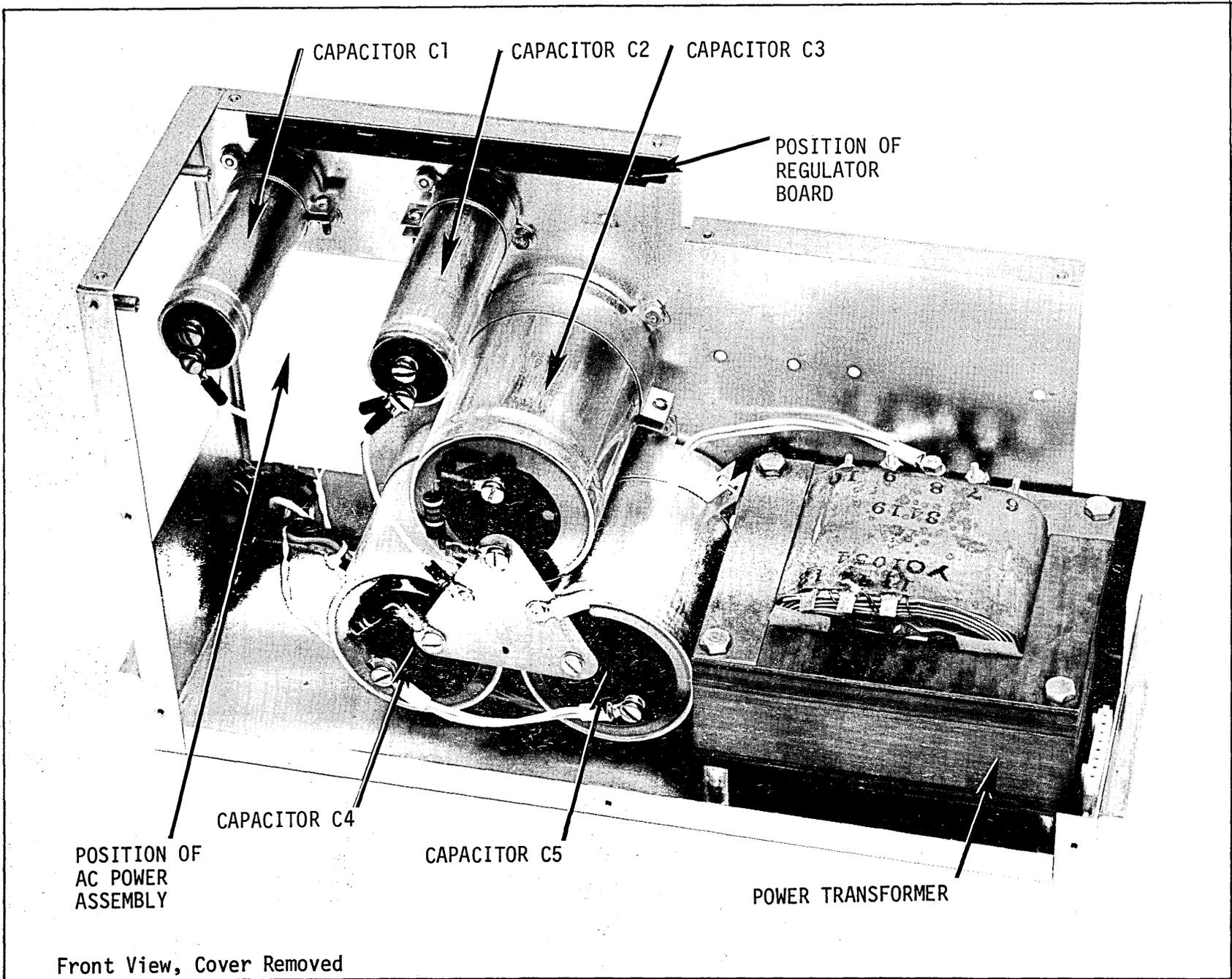
Figure 3-3. 36-A Power Supply Chassis Assembly
